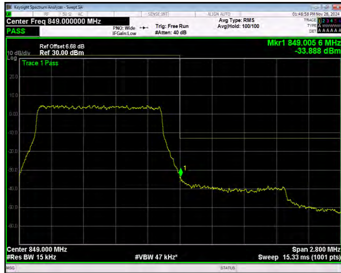
Band26(824-849) QPSK BW=10MHz Channel=26840 RB Size=1 Position=#0 Extended
