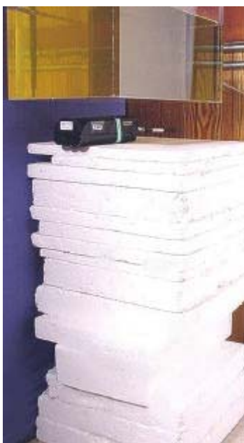
Face-held SAR Test Setup
