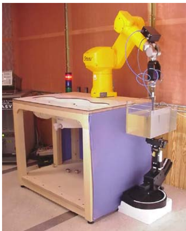
DASY3 SAR Measurement System with Small Planar Phantom
