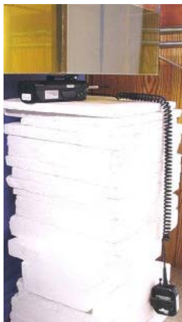
Body-worn SAR Test Setup
