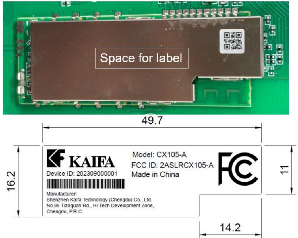
Figure 6 - CX105-A Kaifa radio module mounted on LVM G3 Hybrid GL0
