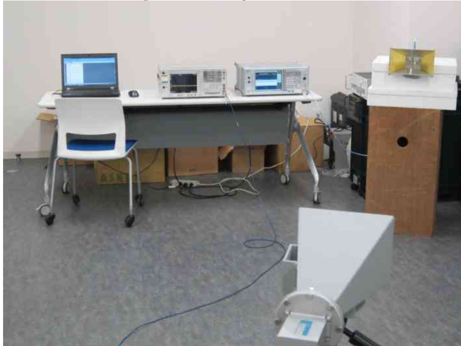
Test Setup for Generating the Radar Waveform
