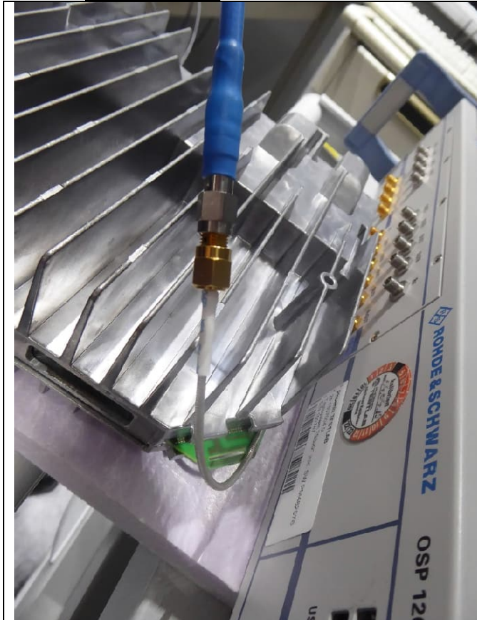
Internal antenna: Temporary antenna connector
