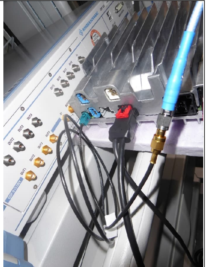
External antenna: Fakra-to-SMA cable
