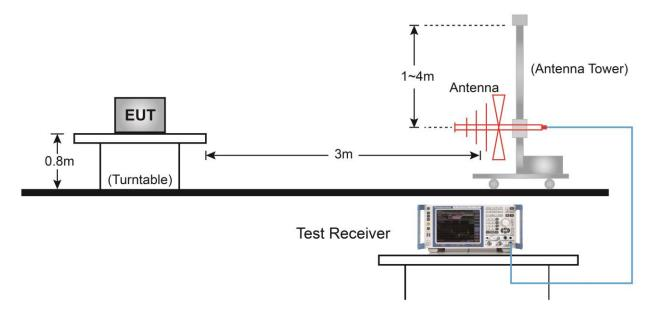
Above 1GHz Test Setup:
