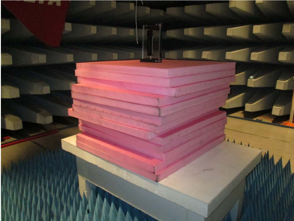
Photo 4.3.1 Test setup regarding measurement of radiated emission. 1-18 GHz.
