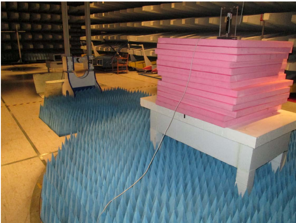
Photo 4.3.2 Test setup regarding measurement of radiated emission 1-18 GHz.
