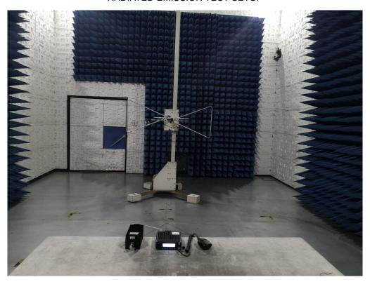
RADIATED EMISSION ABOVE 1G TEST SETUP
