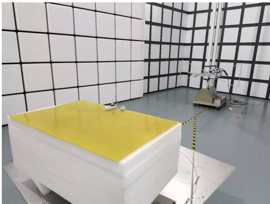
Photo of Radiated Emission Measurement (Above 1G)
