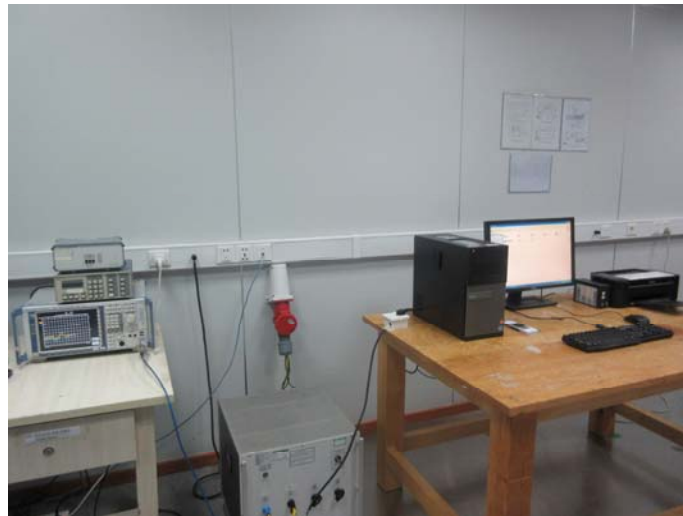
Radiated Emission (30MHz-1GHz) PC Data Transfer
