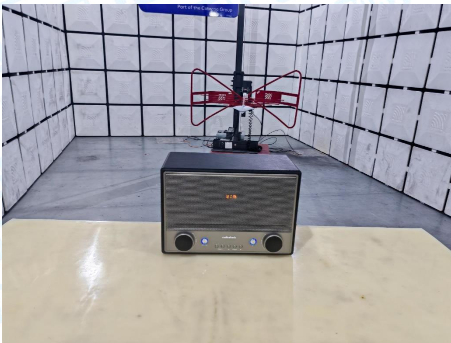
Photo of Setup for Radiated Emission (30MHz~1GHz)
