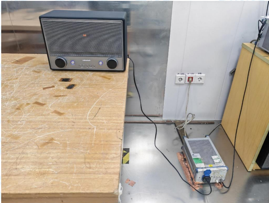
Photo of Setup for Radiated Emission (30MHz~1GHz)
