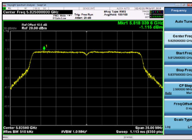
U-NII-3 Power spectral density-802.11 ac(40MHz),5795MHz
