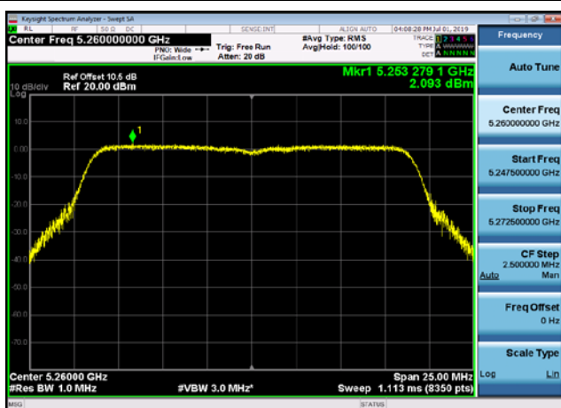
U-NII-2a Power spectral density-802.1 1ac(20MHz),5260MHz
