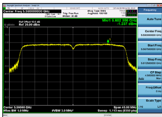
U-NII-2c Power spectral density-802.1 1ac(40MHz),5590MHz
