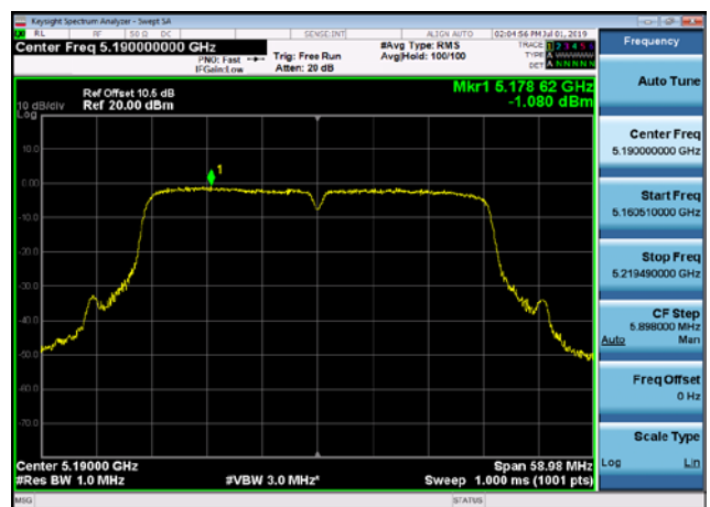
U-NII-1 Power spectral density-802.11 ac(40MHz),5190MHz
