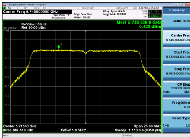
U-NII-3 Power spectral density-802.11 ac(20MHz),5825MHz
