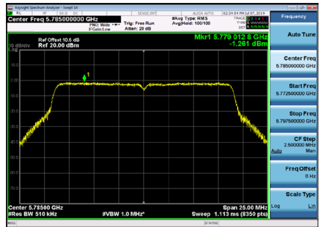
U-NII-3 Power spectral density-802.11 ac(40MHz),5755MHz
