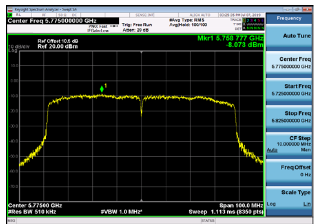
U-NII-3 Power spectral density-802.11 ac(80MHz),5775MHz
