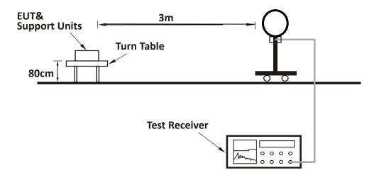
For Radiated emission 30MHz to 1GHz:
