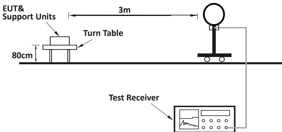
For Radiated emission 30MHz to 1GHz:
