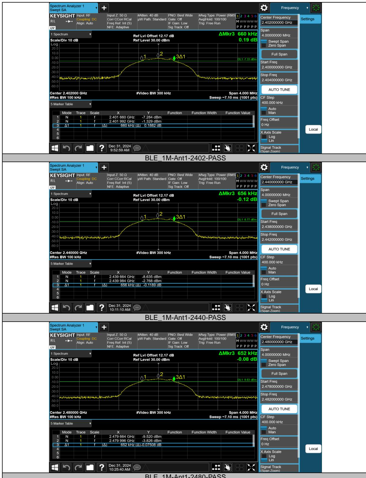
**TEST REPORT****Occupied Channel Bandwidth****Test Result**
