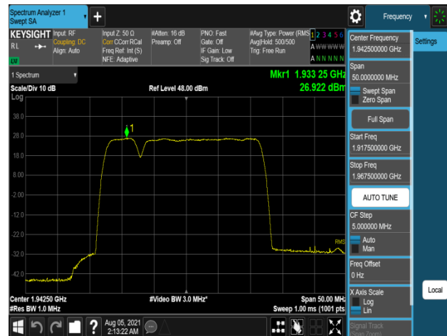
Plot 7-592. Peak Power Spectral Density Plot (B2_5M+20M_2C_16QAM - Low Channel, Port 3)
