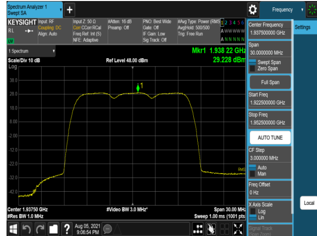
Plot 7-614. Peak Power Spectral Density Plot (B2_5M+5M+5M_3C_16QAM - Low Channel, Port 1)
