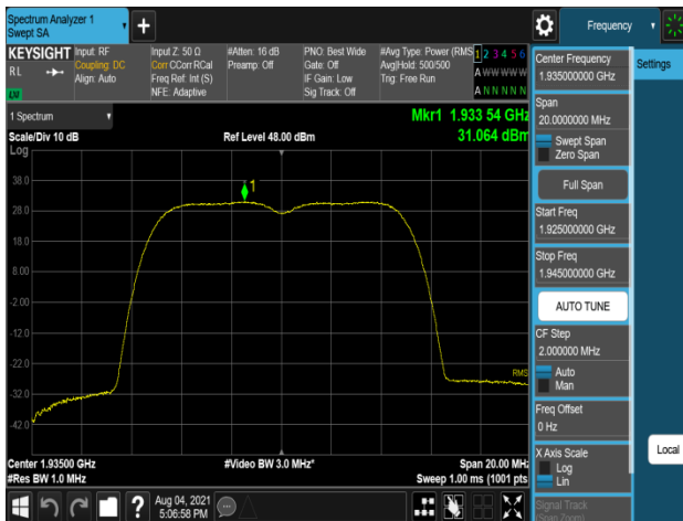
Plot 7-579. Peak Power Spectral Density Plot (B2_5M+5M_2C_16QAM - Low Channel, Port 2)
