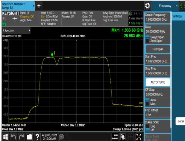
Plot 7-589. Peak Power Spectral Density Plot (B2_5M+20M_2C_16QAM - Low Channel, Port 0)
