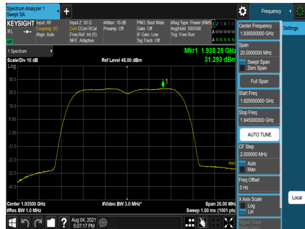
Plot 7-580. Peak Power Spectral Density Plot (B2_5M+5M_2C_16QAM - Low Channel, Port 3)
