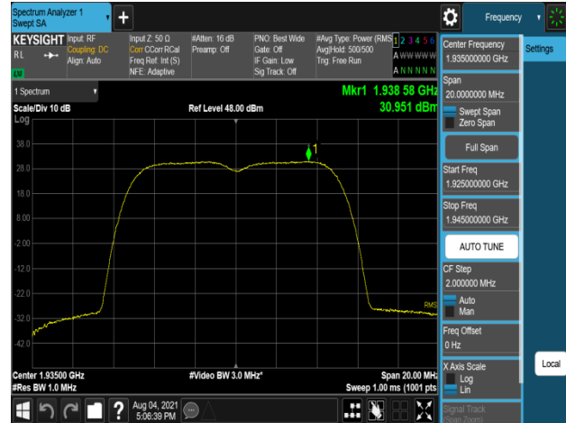
Plot 7-578. Peak Power Spectral Density Plot (B2_5M+5M_2C_16QAM - Low Channel, Port 1)
