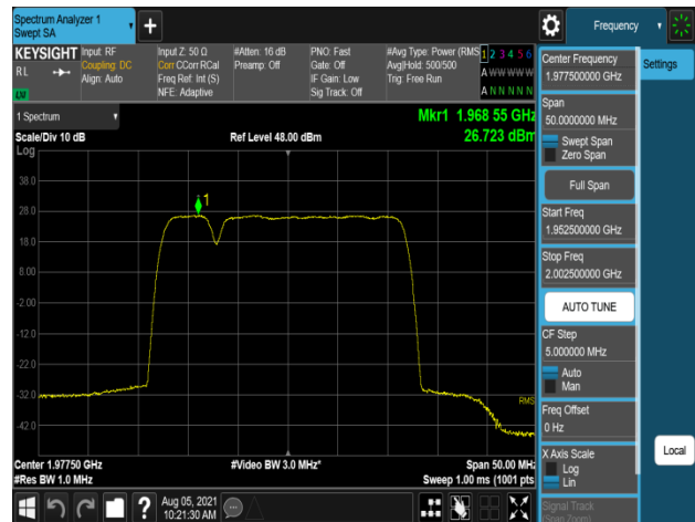
Plot 7-598. Peak Power Spectral Density Plot (B2_5M+20M_2C_16QAM - High Channel, Port 1)
