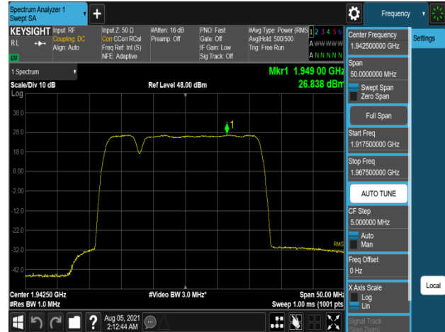
Plot 7-590. Peak Power Spectral Density Plot (B2_5M+20M_2C_16QAM - Low Channel, Port 1)
