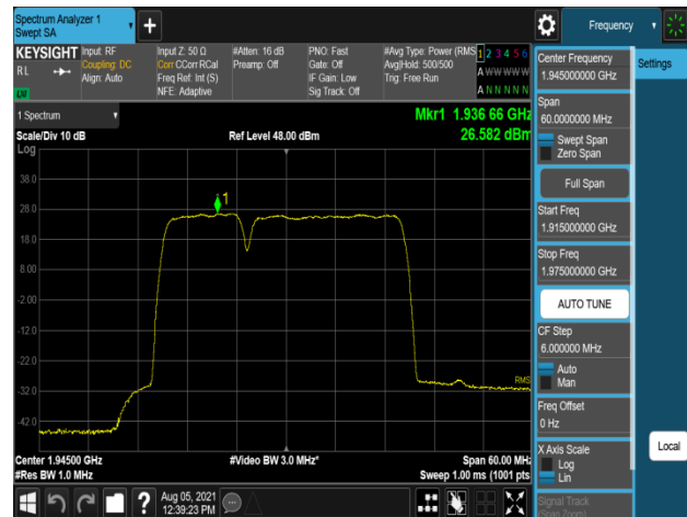
Plot 7-604. Peak Power Spectral Density Plot (B2_10M+20M_2C_16QAM - Low Channel, Port 3)
