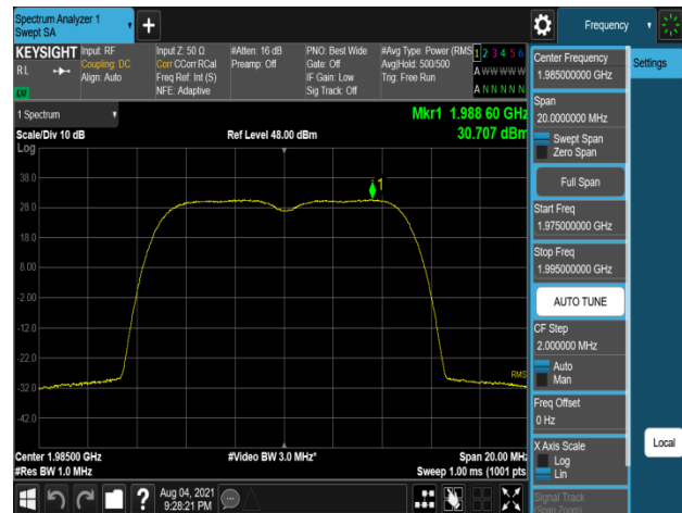
Plot 7-586. Peak Power Spectral Density Plot (B2_5M+5M_2C_16QAM - High Channel, Port 1)
