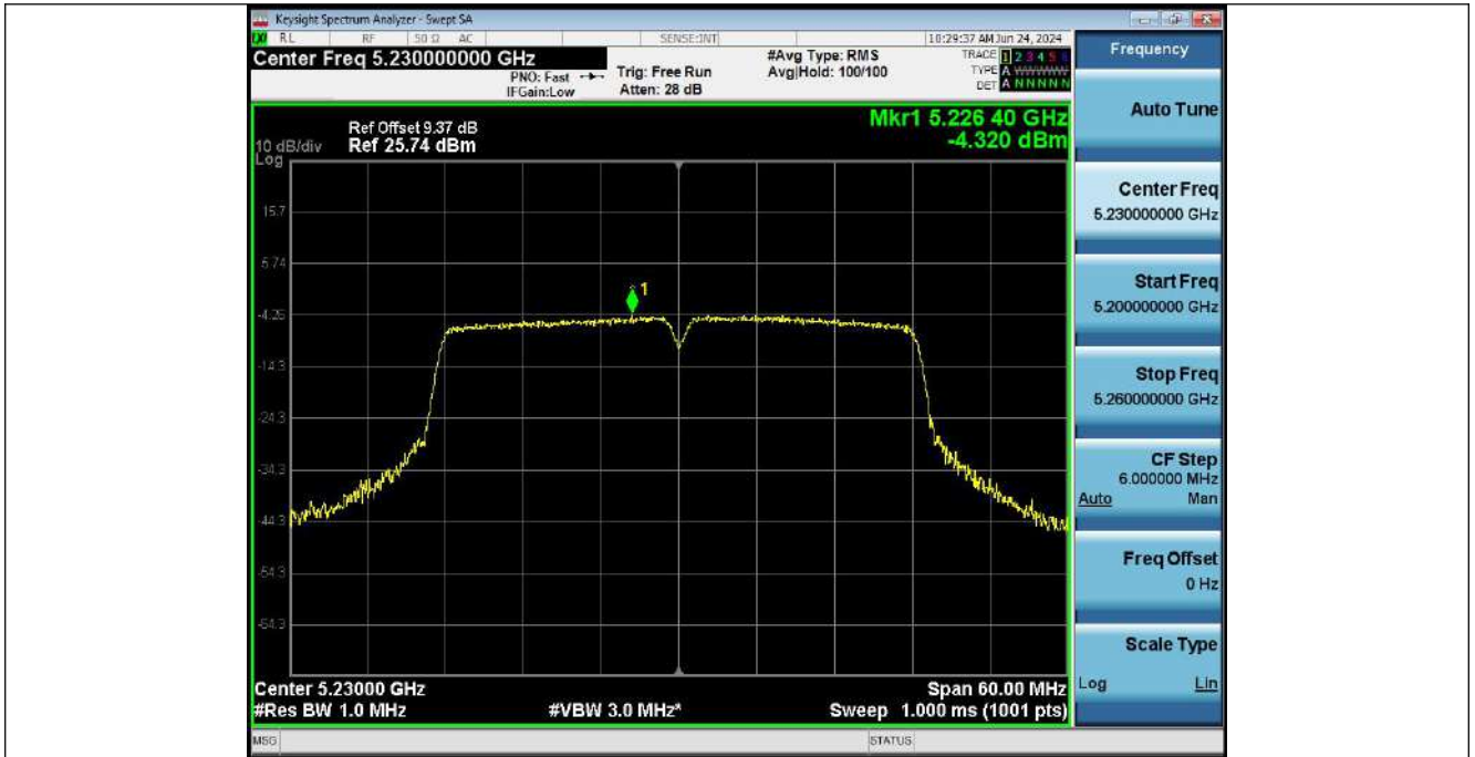
Power Spectral Density_NVNT_ANT1_802_11ax(HE40)_5190
