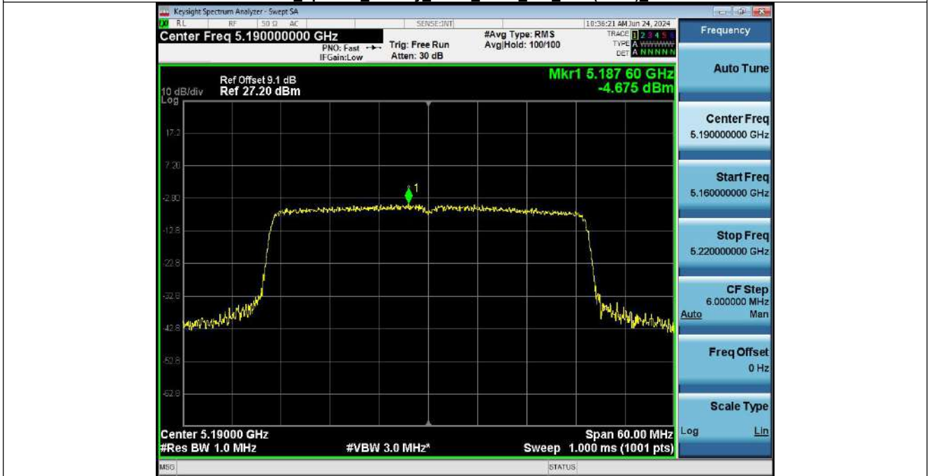
Power Spectral Density_NVNT_ANT1_802_11ax(HE40)_5190
