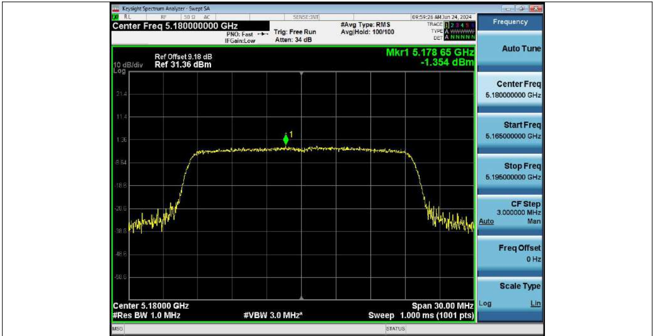
Power Spectral Density_NVNT_ANT1_802_11ax(HE20)_5200
