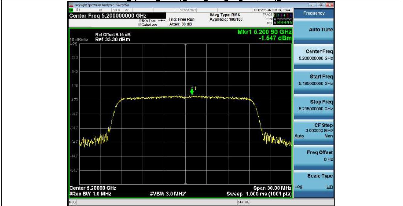
Power Spectral Density_NVNT_ANT1_802_11ax(HE20)_5200
