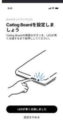
Press the [LED flashing blue] button to start searching for the Board.
