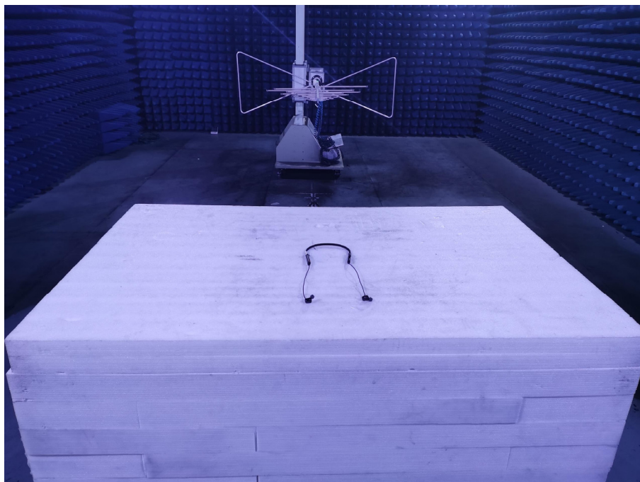
Photo of Radiated Emission Measurement (Above 1G)
