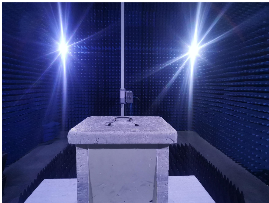
Photo of Radiated Emission Measurement (Above 1G)
