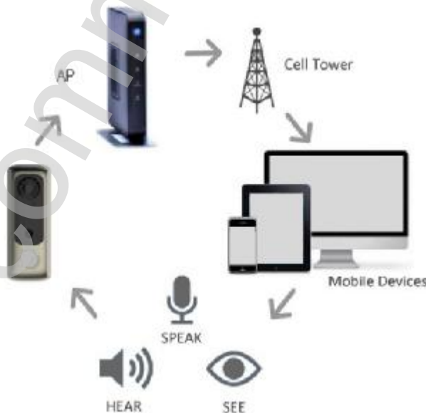
Figure 1: Network Diagram - Wireless HD Doorbell Camera
