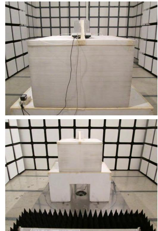
Test Mode 3: EUT 1 + Set 3 Sector Antenna / 5.5 dBi
