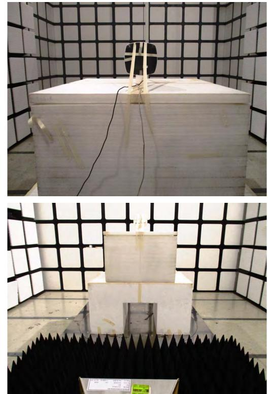
Mode 7: EUT 2 + Set 10 PIFA Antenna / Chain1:3.81 dBi, Chain2:3.75 dBi, Chain3:3.98 dBi, Chain4:3.47 dBi
