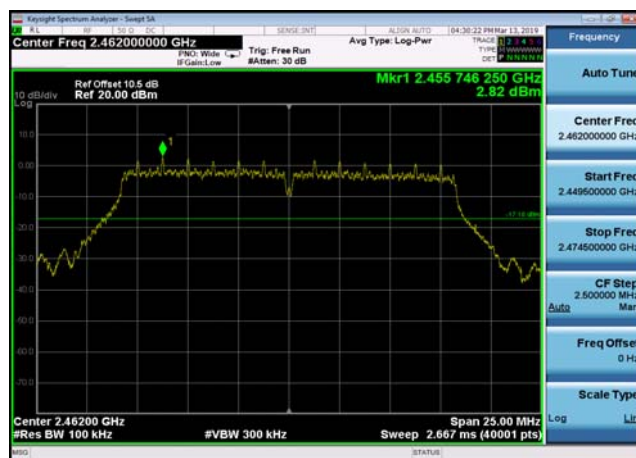
,Plot 1,Reference Level-802.11g ,2462MHz
