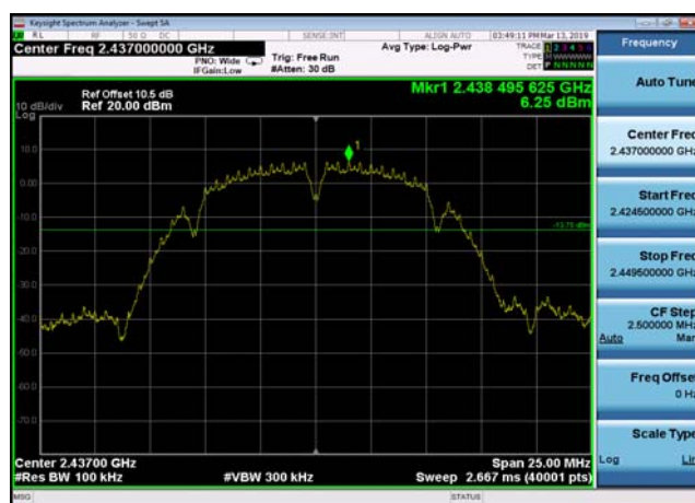
,Plot 2,Band Edge-802.11b,2412MHz
