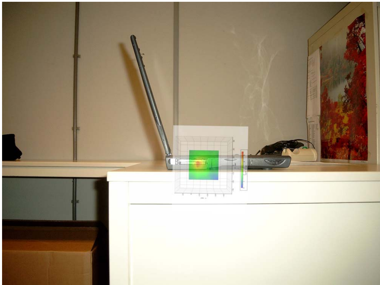
Photo 5: A 2d scan overlay giving the field strength in the first scanned plane, overlaid on a side view photo of the laptop. 2d scan is that of the worst case perpendicular value in channel 147.
