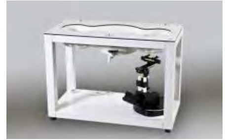
Figure 3.6 SAM Twin Phantom
