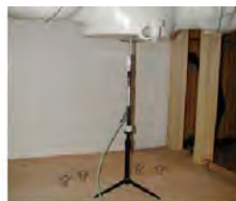
Figure 11.1 Dipole Verification Test Setup Diagram & Photo
