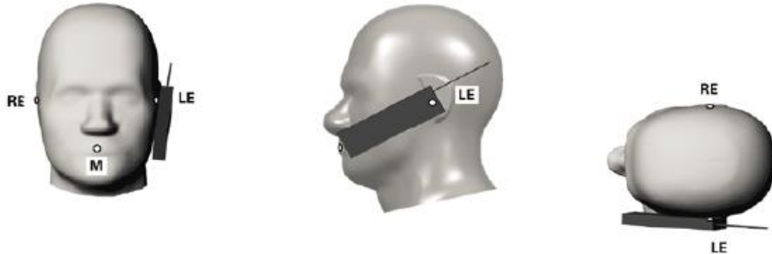
Fig. 11.3 Illustration for Cheek Position
