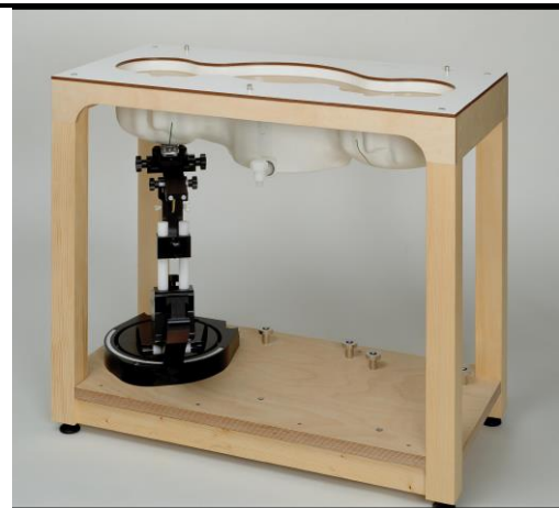
Fig. 8.7 Photo of SAM Twin Phantom
