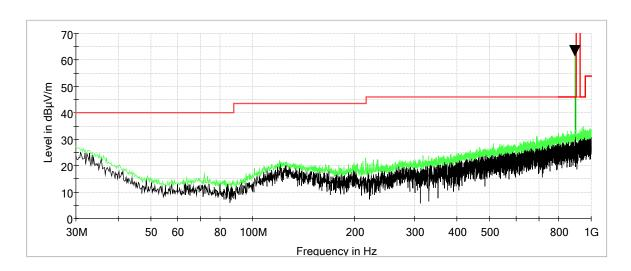
Note: The 900 MHz emission is a separate transmitter, refer to F2 Labs Report F2P30751A-R1-01E.
