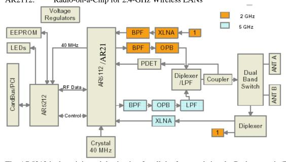
The AR5212 is the origin and destination for all the front-end signals. Both transmit (Tx) and receive (Rx) signals are transferred by the AR5112 to either a 5GHz front-end, or a 2.4GHz front end.
