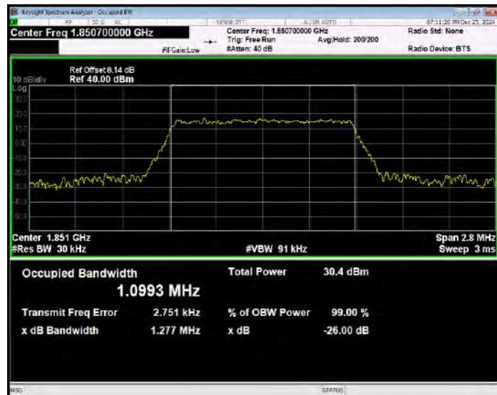
Band2 QPSK BW=1.4MHz Channel=18900 RB Size=6 Position=#0
