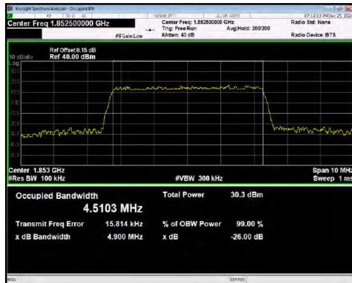
Band2 QPSK BW=5MHz Channel=18900 RB Size=25 Position=#0
