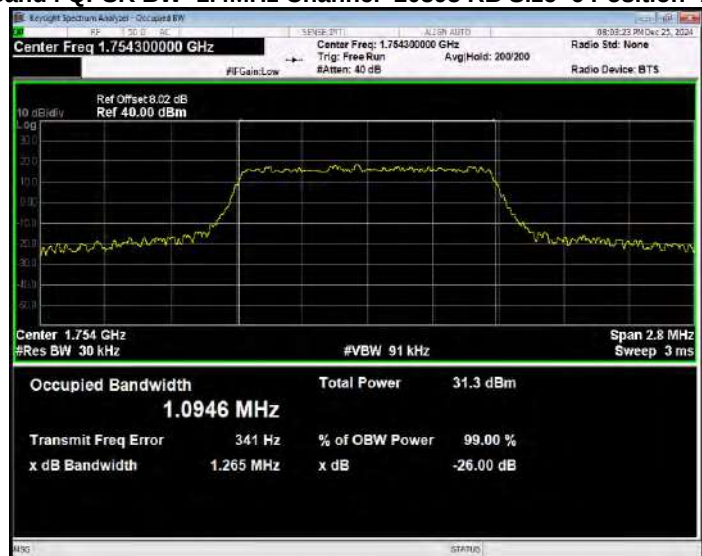
Band4 QPSK BW=10MHz Channel=20000 RB Size=50 Position=#0
