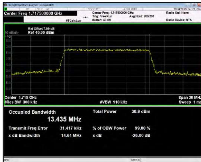
Band4 QPSK BW=15MHz Channel=20175 RB Size=75 Position=#0
