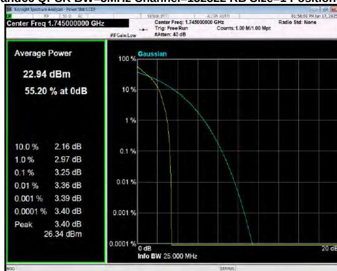
Band66 QPSK BW=3MHz Channel=132657 RB Size=1 Position=#0
