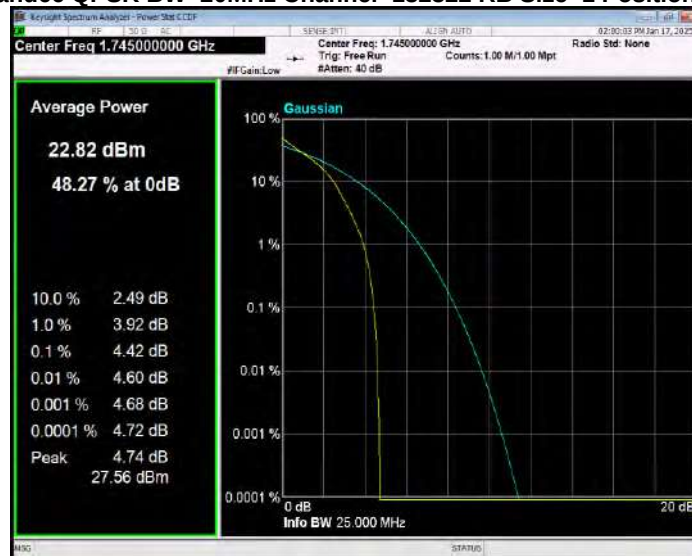
Band66 QPSK BW=20MHz Channel=132572 RB Size=1 Position=#0
