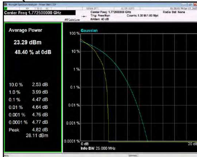
Band66 QPSK BW=20MHz Channel=132072 RB Size=1 Position=#0
