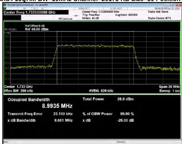
Band4 16QAM BW=10MHz Channel=20350 RB Size=50 Position=#0
