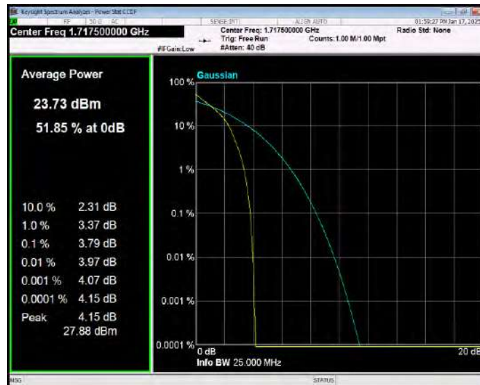
Band66 QPSK BW=15MHz Channel=132322 RB Size=1 Position=#0
