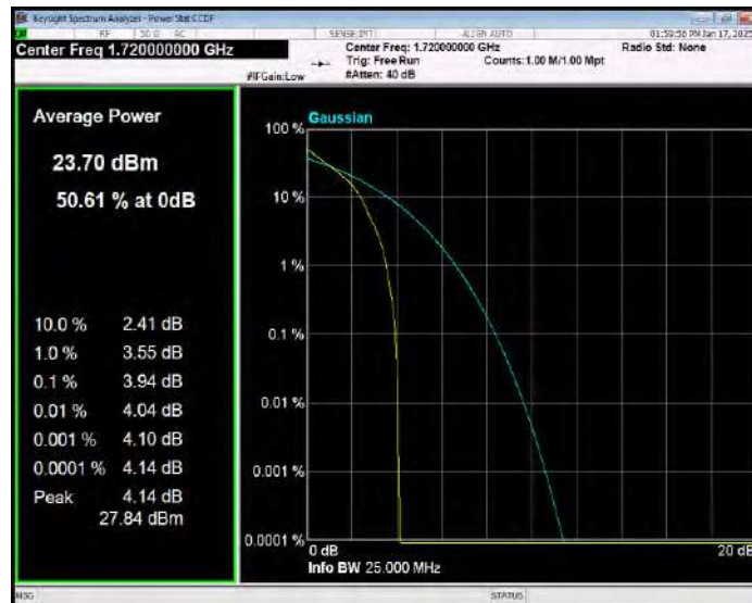
Band66 QPSK BW=20MHz Channel=132322 RB Size=1 Position=#0
