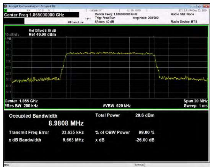
Band2 QPSK BW=10MHz Channel=18900 RB Size=50 Position=#0
