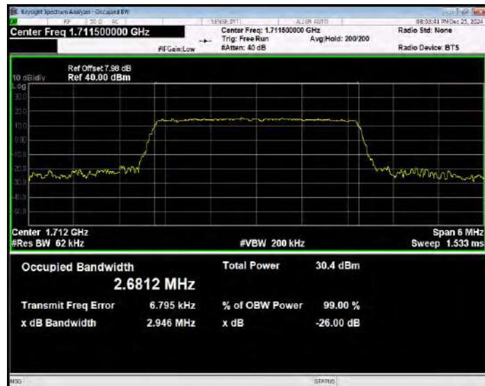
Band4 16QAM BW=3MHz Channel=20175 RB Size=15 Position=#0
