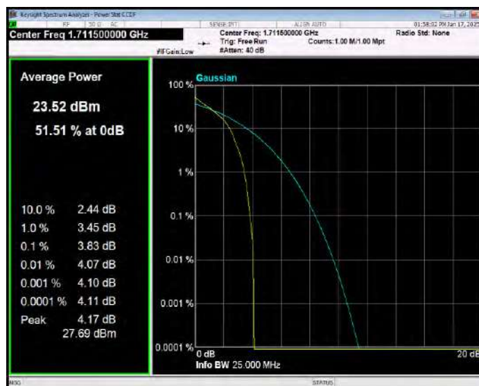
Band66 QPSK BW=3MHz Channel=132322 RB Size=1 Position=#0
