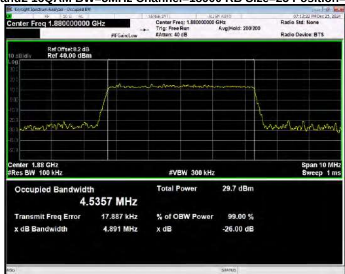
Band2 16QAM BW=5MHz Channel=19175 RB Size=25 Position=#0
