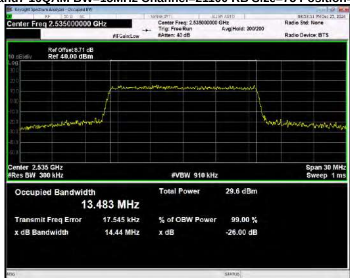
Band7 16QAM BW=15MHz Channel=21375 RB Size=75 Position=#0
