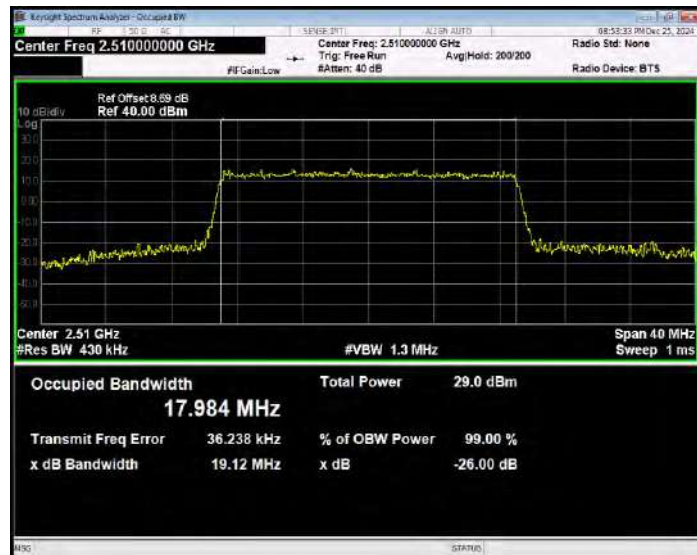
Band7 16QAM BW=20MHz Channel=21100 RB Size=100 Position=#0
