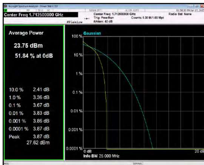
Band66 QPSK BW=5MHz Channel=132322 RB Size=1 Position=#0
