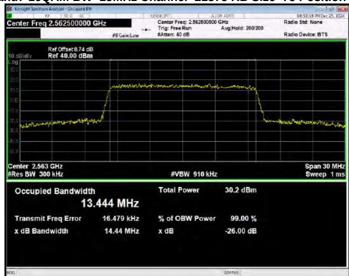
Band7 16QAM BW=20MHz Channel=20850 RB Size=100 Position=#0
