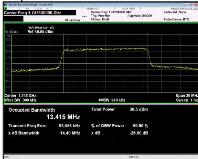
Band4 QPSK BW=20MHz Channel=20050 RB Size=100 Position=#0
