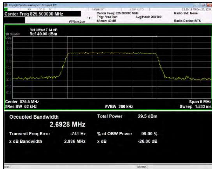
Band5 16QAM BW=3MHz Channel=20525 RB Size=15 Position=#0
