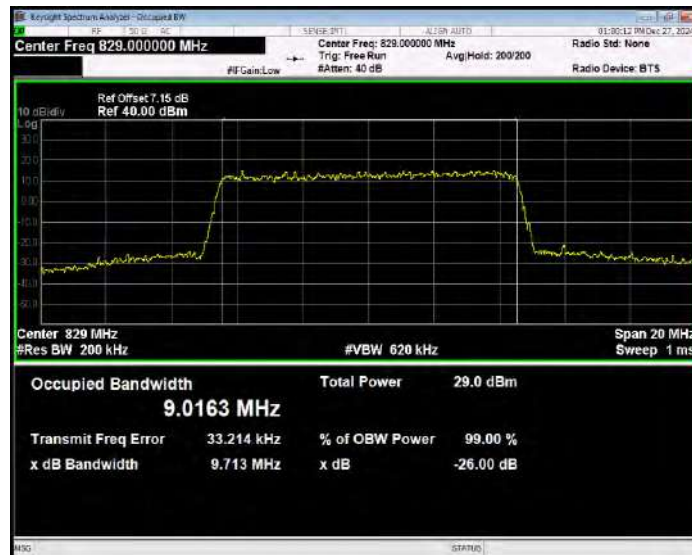
Band5 16QAM BW=10MHz Channel=20525 RB Size=50 Position=#0
