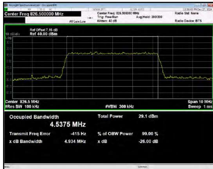
Band5 16QAM BW=5MHz Channel=20525 RB Size=25 Position=#0
