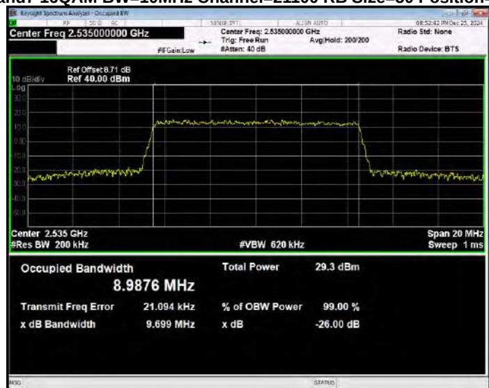
Band7 16QAM BW=10MHz Channel=21400 RB Size=50 Position=#0
