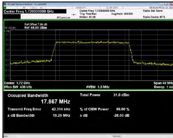
Band4 QPSK BW=20MHz Channel=20175 RB Size=100 Position=#0
