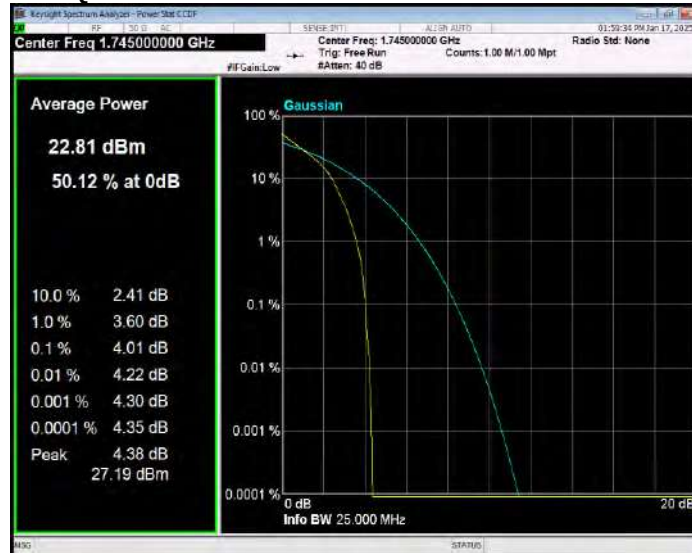
Band66 QPSK BW=15MHz Channel=132597 RB Size=1 Position=#0
