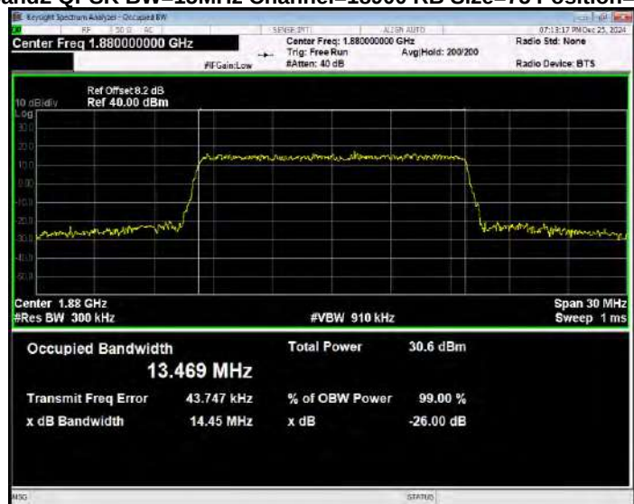
Band2 QPSK BW=15MHz Channel=19125 RB Size=75 Position=#0
