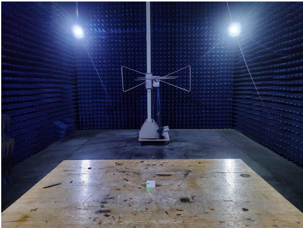
Photo of Radiated Emission Measurement (Below 1G)
