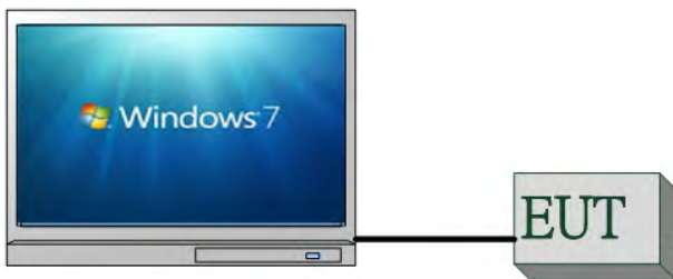
Fig. 2-2 Conducted Emission Configuration
