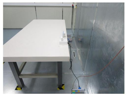
Test Mode: Mode1 with Adapter (2) Description: Front View of Conducted Emission Test Setup
