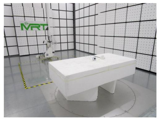
Test Mode: Mode 1 Description: Radiated Emission Test Setup for above 1GHz
