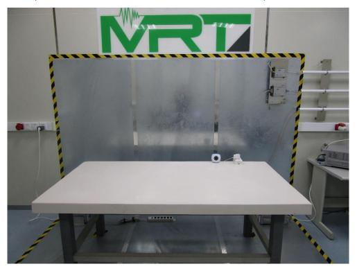
Test Mode: Mode1 with Adapter (2) Description: Back View of Conducted Emission Test Setup
