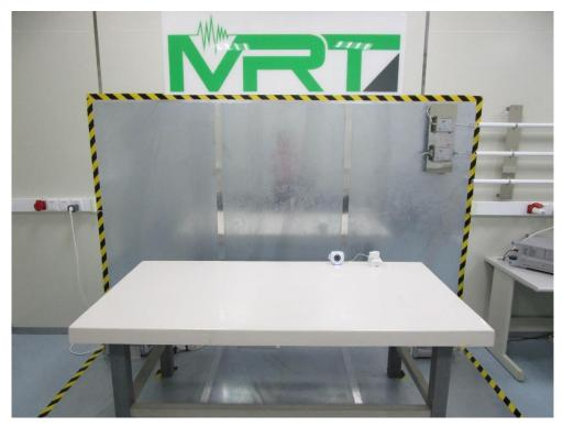
Test Mode: Mode1 with Adapter (1) Description: Back View of Conducted Emission Test Setup
