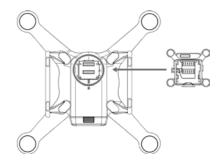
Slide the Quick-mount Module onto the Quick-mount Base towards the Lock direction ( ) indicated beside the Unlock button. You will hear a clicking sound when the gimbal is properly installed.
