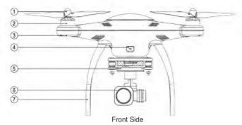
1) Propeller 2 Motor ③ Front LED Indicator Light ( 1 5) (4) Micro-USB Port
