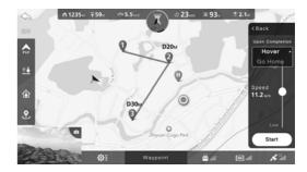
**3.** Set a safe altitude for the aircraft to perform **Go Home** at low battery level.
