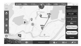
Draw on Map - Select Draw on Map from the drop-down box of Waypoint Location and your screen will be switched to the map. Move your finger to draw a route on the map, and the waypoints will be identified automatically according to your route. The Clear Waypoints button is used to delete the entire route. When you have confirmed your route, tap Finish.
