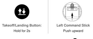
If you command the aircraft to take off using 11, the aircraft will ascend automatically to a height of 4 meters.
