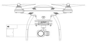
Reinstall the gimbal holder after using the aircraft to protect the gimbal from unwanted movements when not in use.
