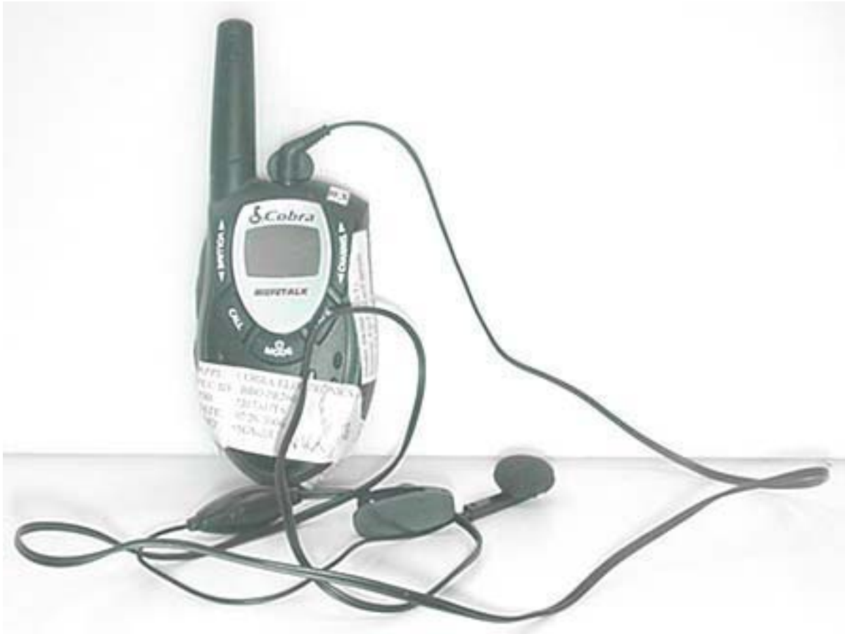
DUT with Earbud Lapel-Microphone Audio Accessory (P/N: GA-EBM2)
