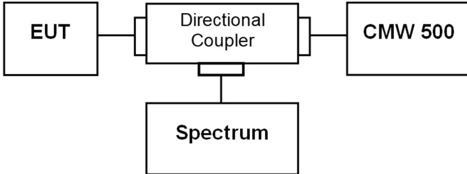
Radiated Spurious Measurement (below 1GHz)
