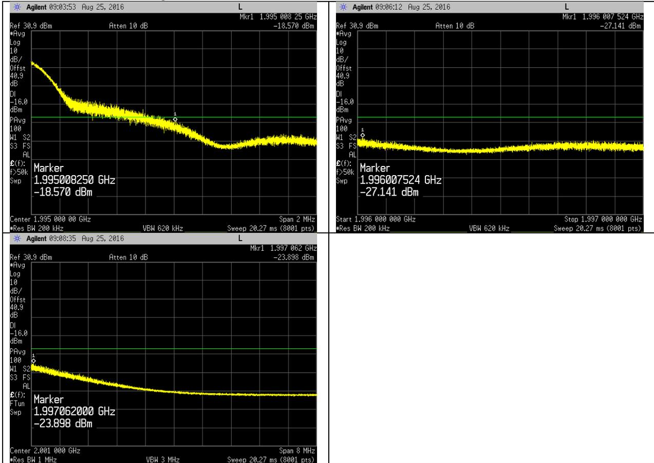
**Transmitter Antenna Port Conducted Spurious Emissions**
