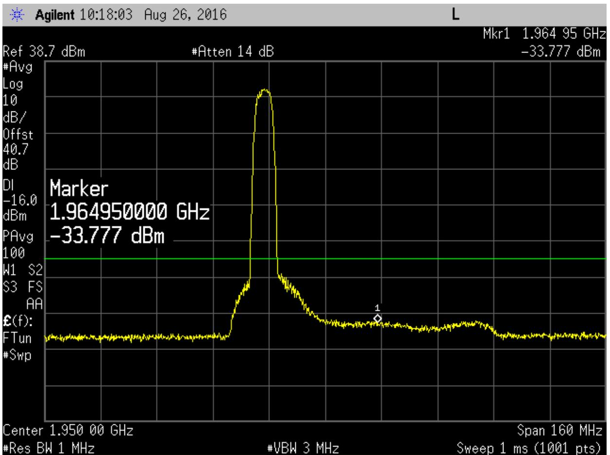
5M - LTE - 16QAM - High Channel
