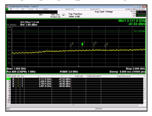
RE\_1 - 5 GHz\_ Band 7\_4 carrier\_\_TX1 and TX2 on at max power.
