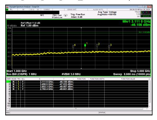
RE\_1 - 5 GHz\_ Band 6\_4 carrier\_\_TX1 and TX2 on at max power.
