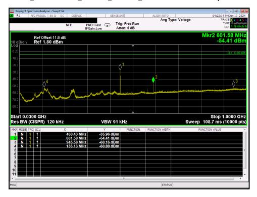
RE\_30 - 1000 MHz\_ Band 6\_4 carrier\_TX1 and TX2 on at max power
