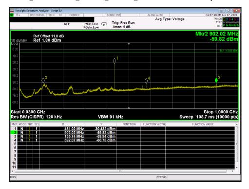
RE\_30 - 1000 MHz\_ Band 5\_4 carrier\_TX1 and TX2 on at max power
