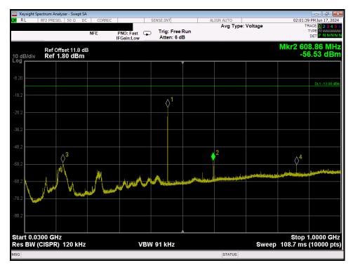
RE\_30 - 1000 MHz\_ Band 7\_4 carrier\_TX1 and TX2 on at max power
