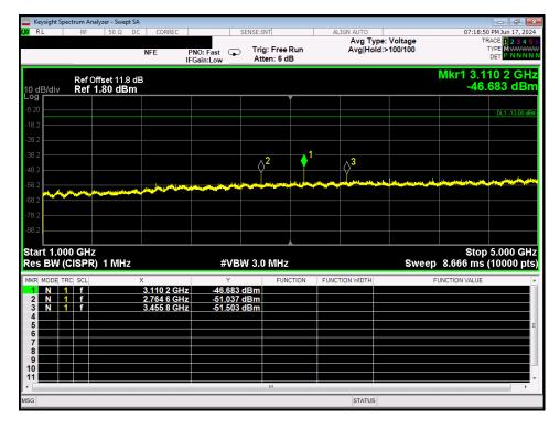
RE\_1 - 5 GHz\_ Band 5\_4 carrier\_\_TX1 and TX2 on at max power.
