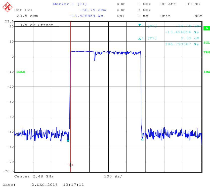
**Pulse time, Low Channel, 2DH3**
