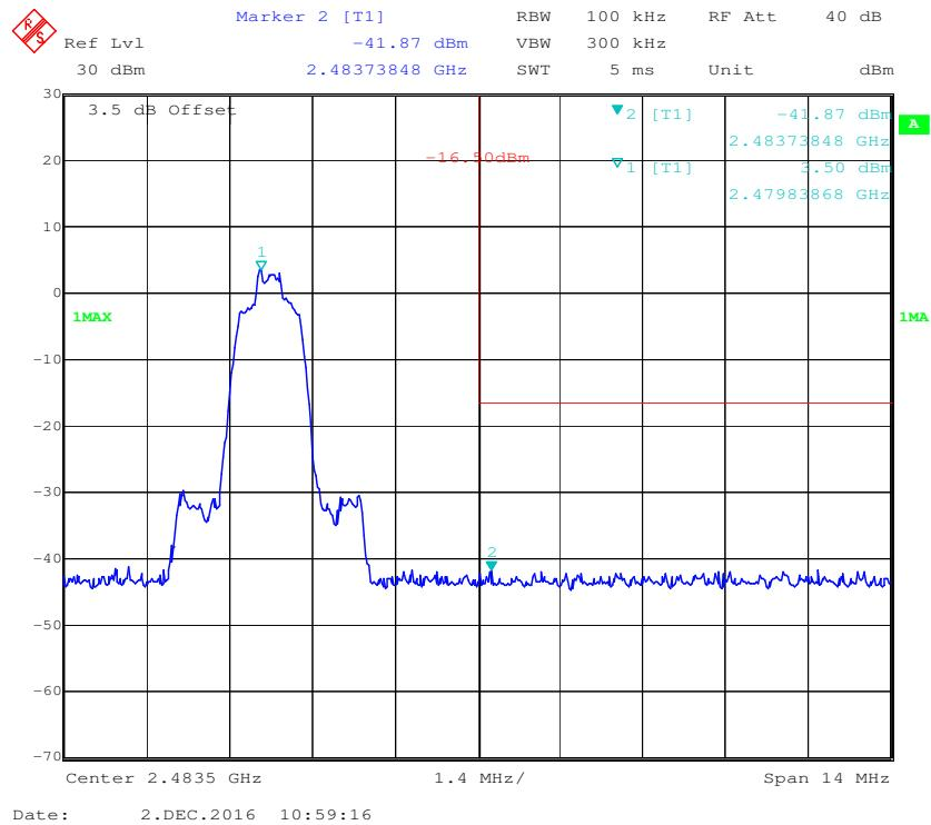
**EDR (8DPSK): Band Edge-Left Side**
