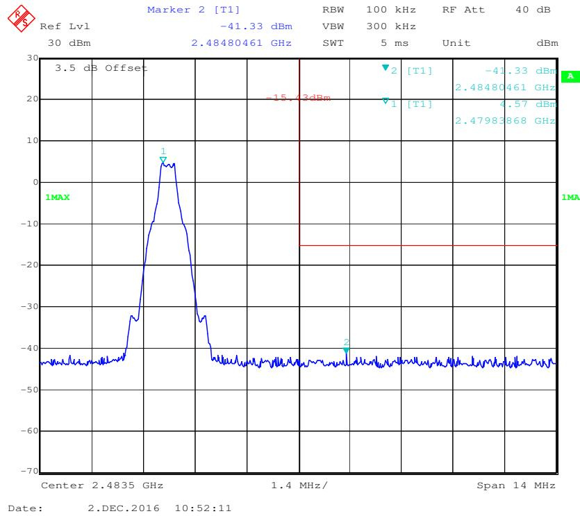
**EDR ( $\pi/4$ -DQPSK): Band Edge-Left Side**
