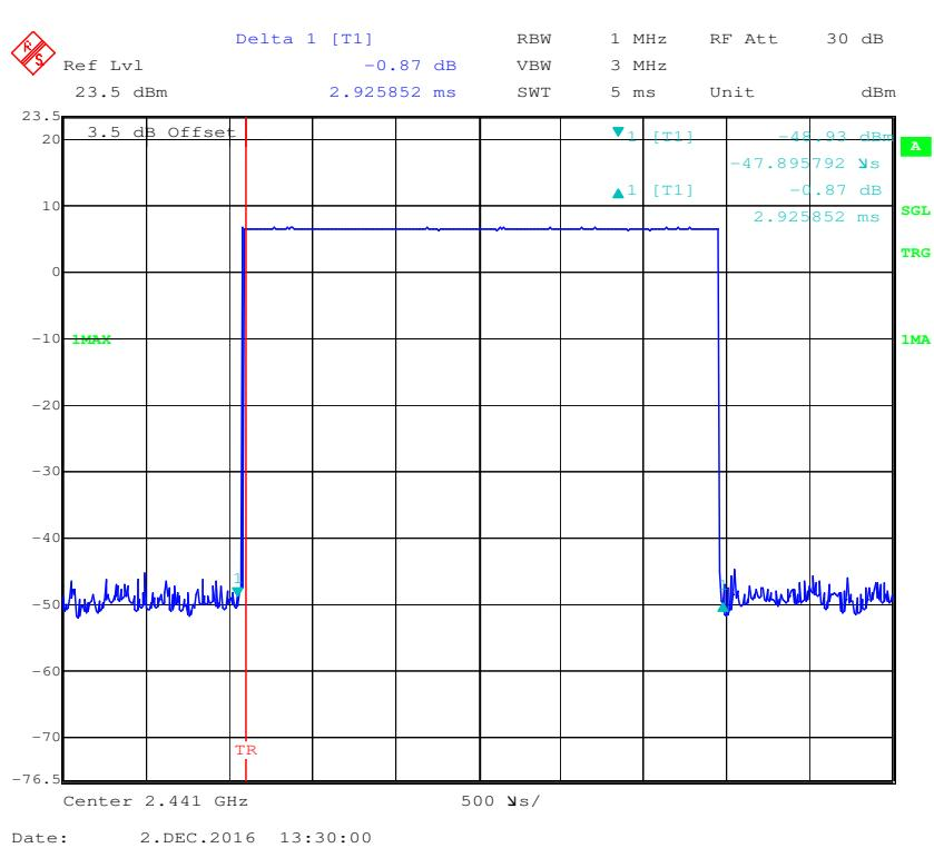
**Pulse time, High Channel, DH5**
