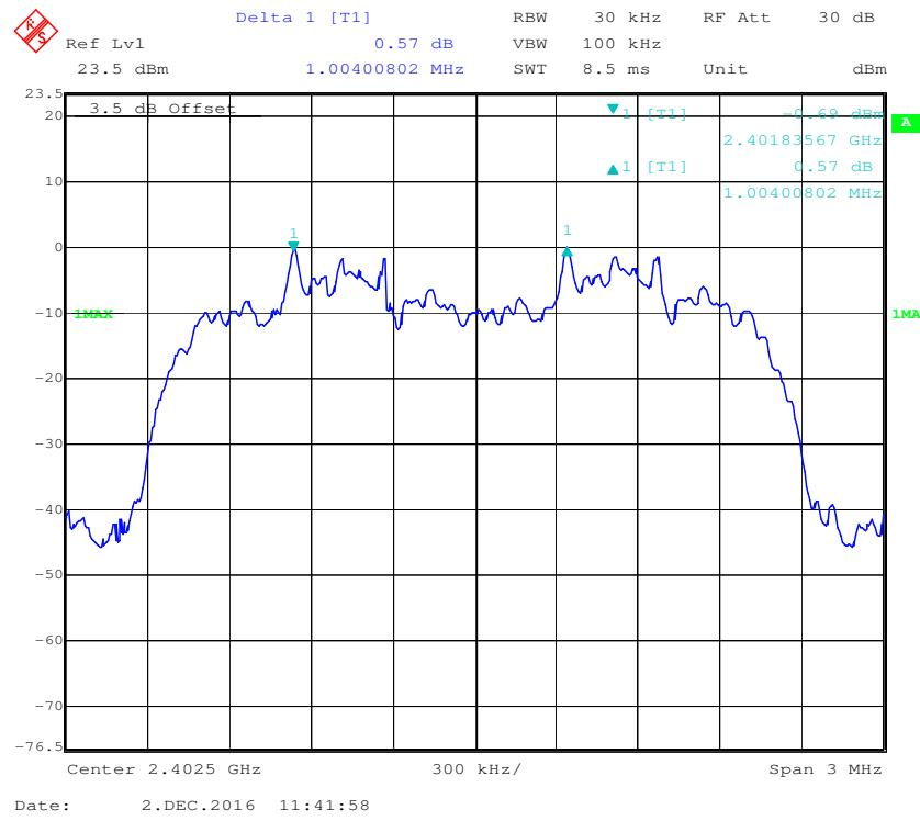
**EDR ( $\pi/4$ -DQPSK): Middle Channel**
