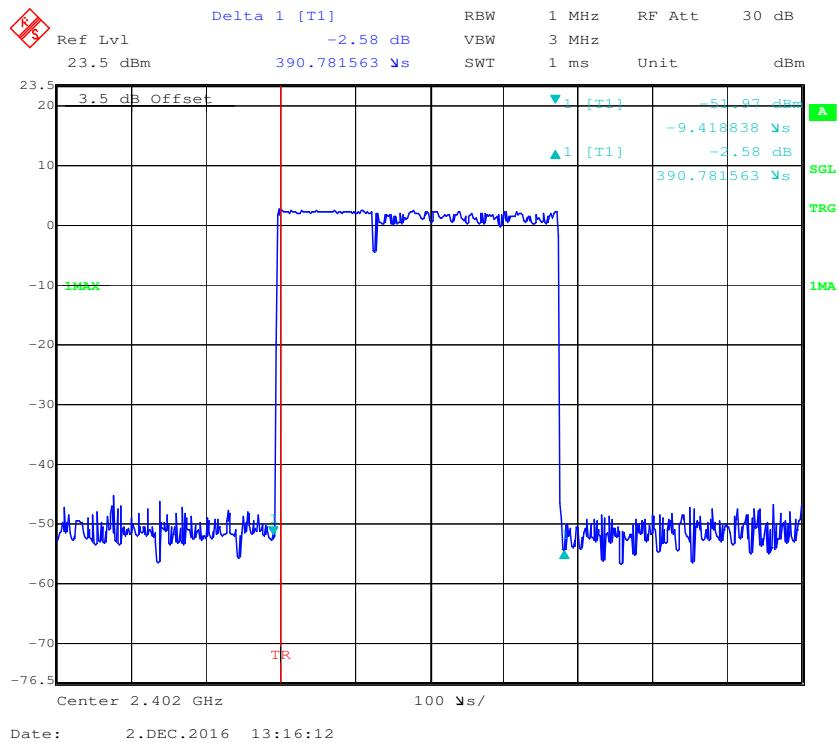
**Pulse time, Middle Channel, 2DH1**
