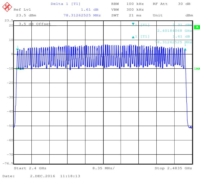
**EDR ( $\pi/4$ -DQPSK): Number of Hopping Channels**
