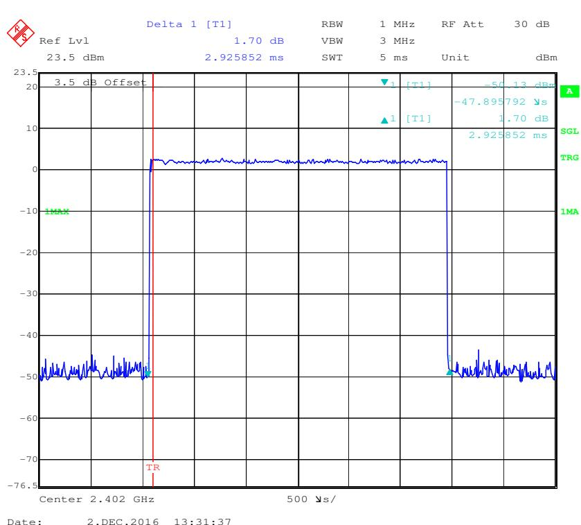
**Pulse time, Middle Channel, 2DH5**
