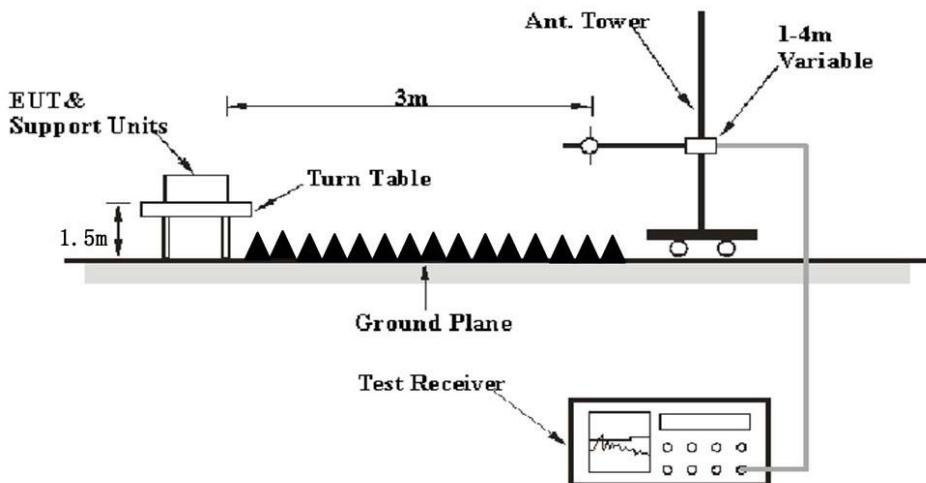
The radiated emission tests were performed in the 3 meters, using the setup accordance with the ANSI ANSI C63.10-2013. The specification used was the FCC 15.209, 205 and FCC 15.247 limits.
