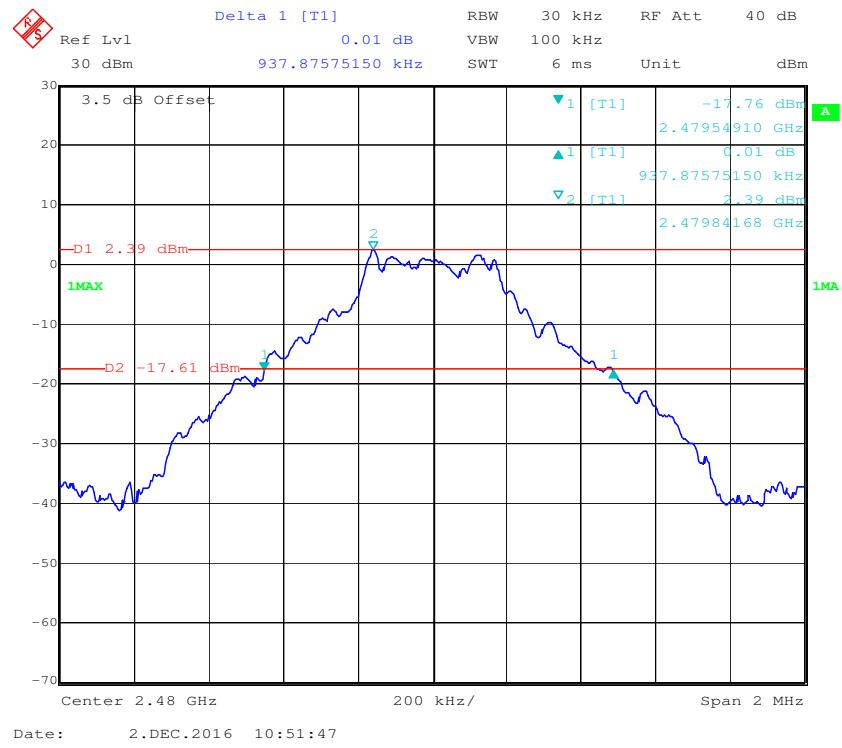
**EDR ( $\pi/4$ -DQPSK): Low Channel**
