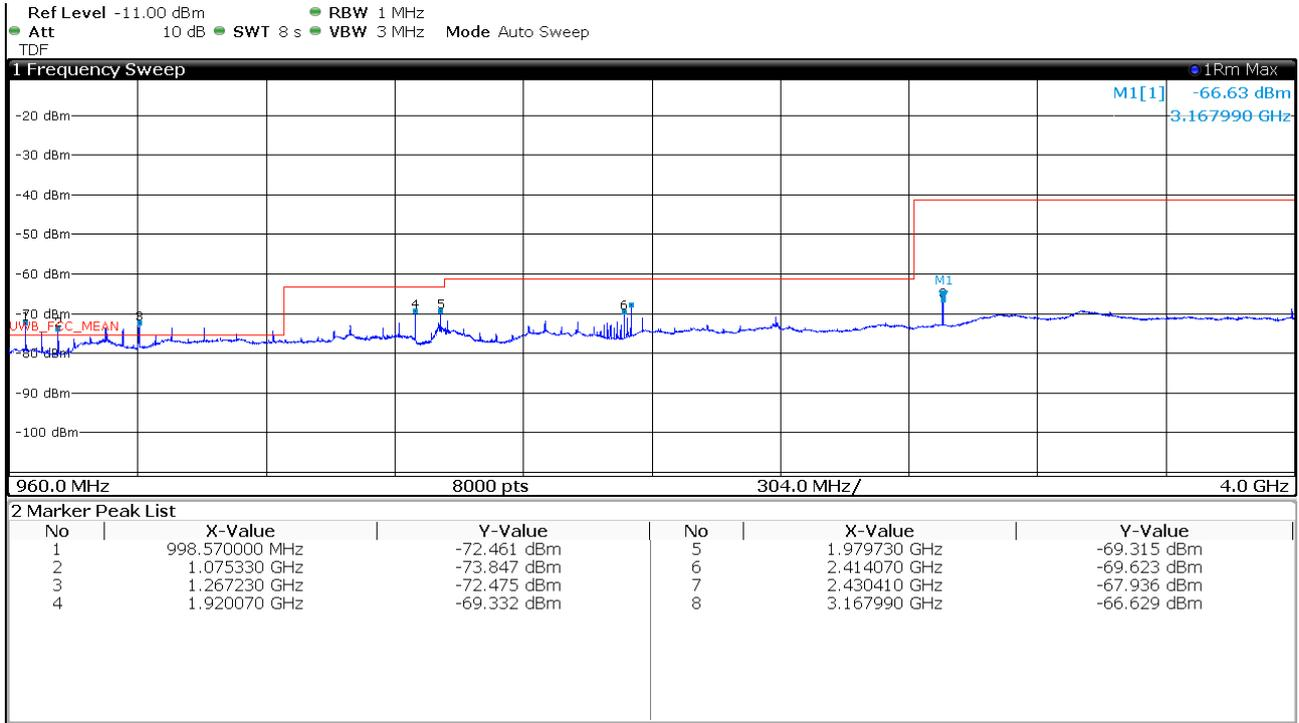
Note: The values above the limit line are not belonging to the UWB technology. These values are considered in the test report T44481-00-07KS of the test laboratory CSA Group Bayern GmbH.
