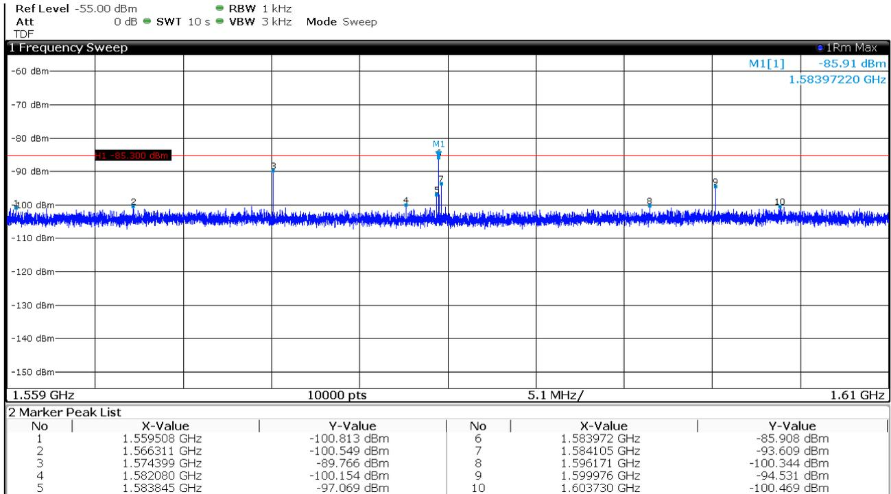
Note: The value above the limit line is not belonging to the UWB technology. This value is considered in the test report T44481-00-07KS of the test laboratory CSA Group Bayern GmbH.
