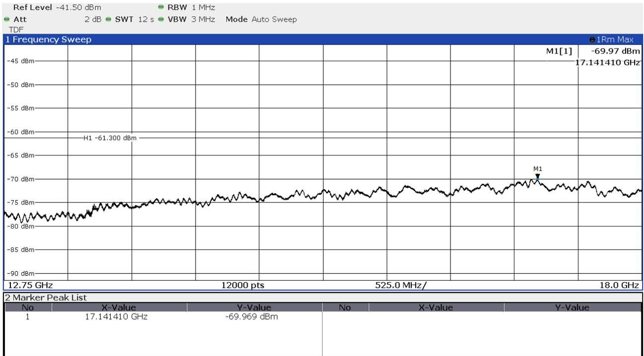
12.75 GHz to 18 GHz with a RBW of 100 kHz at 3 m
