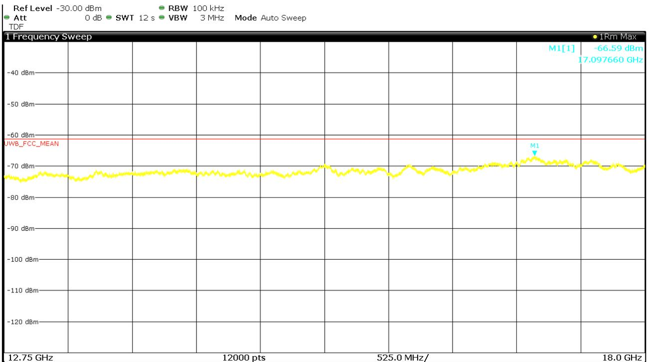
Note: the measurement has also been performed with a resolution bandwidth of 100 kHz to reduce the noise floor and to show that there are no emissions of the device.
