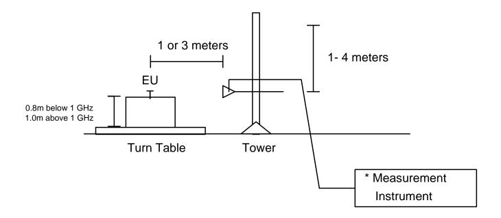
\* 30-1000 MHz, Rohde & Schwarz ESI-40 receiver or 1-10 GHz, R&S ESI-40 with preamplifier and high-pass filter
