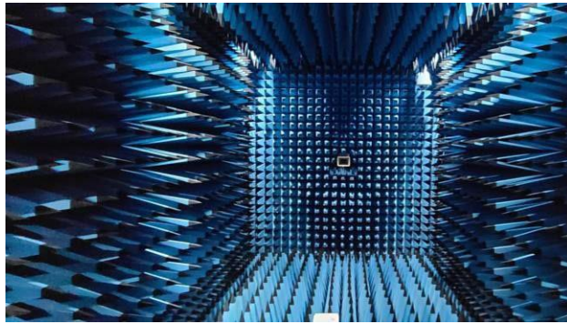
Figure 2: Geometry of Anechoic Chamber for Radiation patterns.
