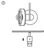
Next take your Apple Watch® Magnetic Charging Cable and put the USB end through the bottom slot on the charging stand.
