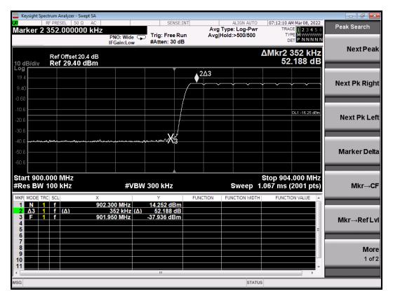
Screen Capture from the spectrum analyzer: Upper Band Edge (Hopping)
