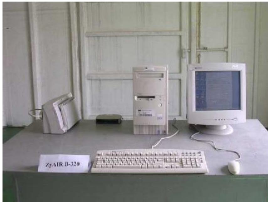
Photo 2: Radiated Emission Test Set-up
