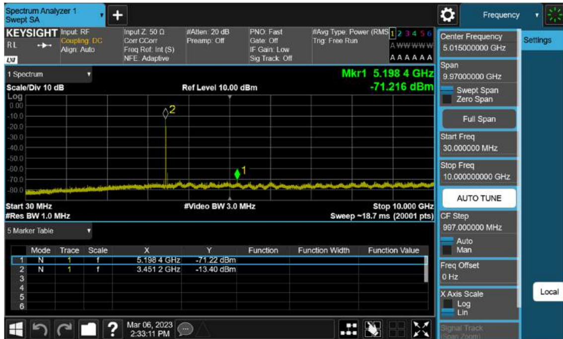
Sub6 n77(78). Conducted Spurious Plot_1 (633334ch_100 MHz_BPSK)
