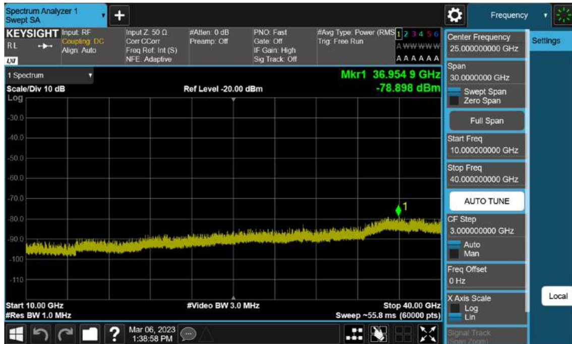
Sub6 n77(78). Conducted Spurious Plot_2 (634332ch_70 MHz_BPSK)
