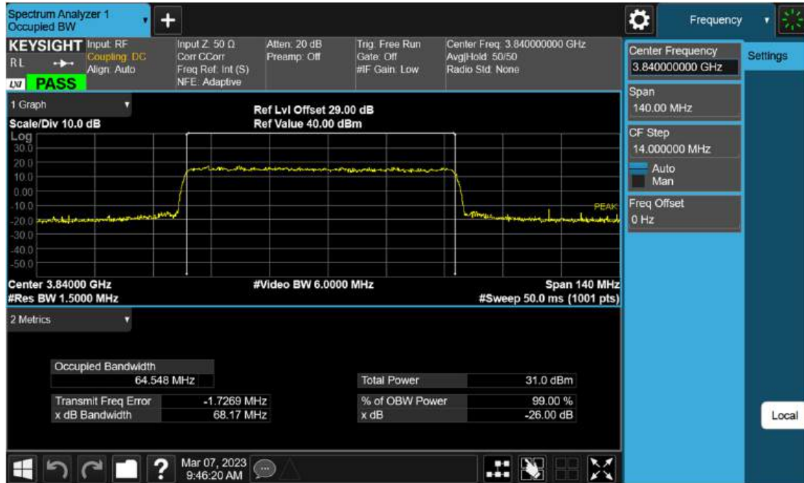
Sub6 n77(78). Occupied Bandwidth Plot (70 M BW Ch.656000 64 QAM )
