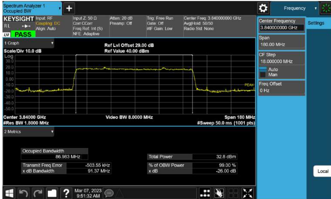
Sub6 n77(78). Occupied Bandwidth Plot (90 M BW Ch.656000 BPSK )
