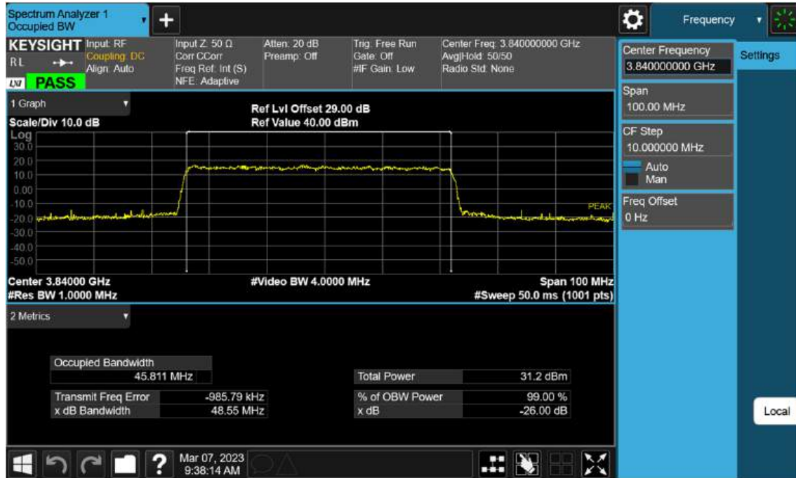
Sub6 n77(78). Occupied Bandwidth Plot (50 M BW Ch.656000 16QAM )
