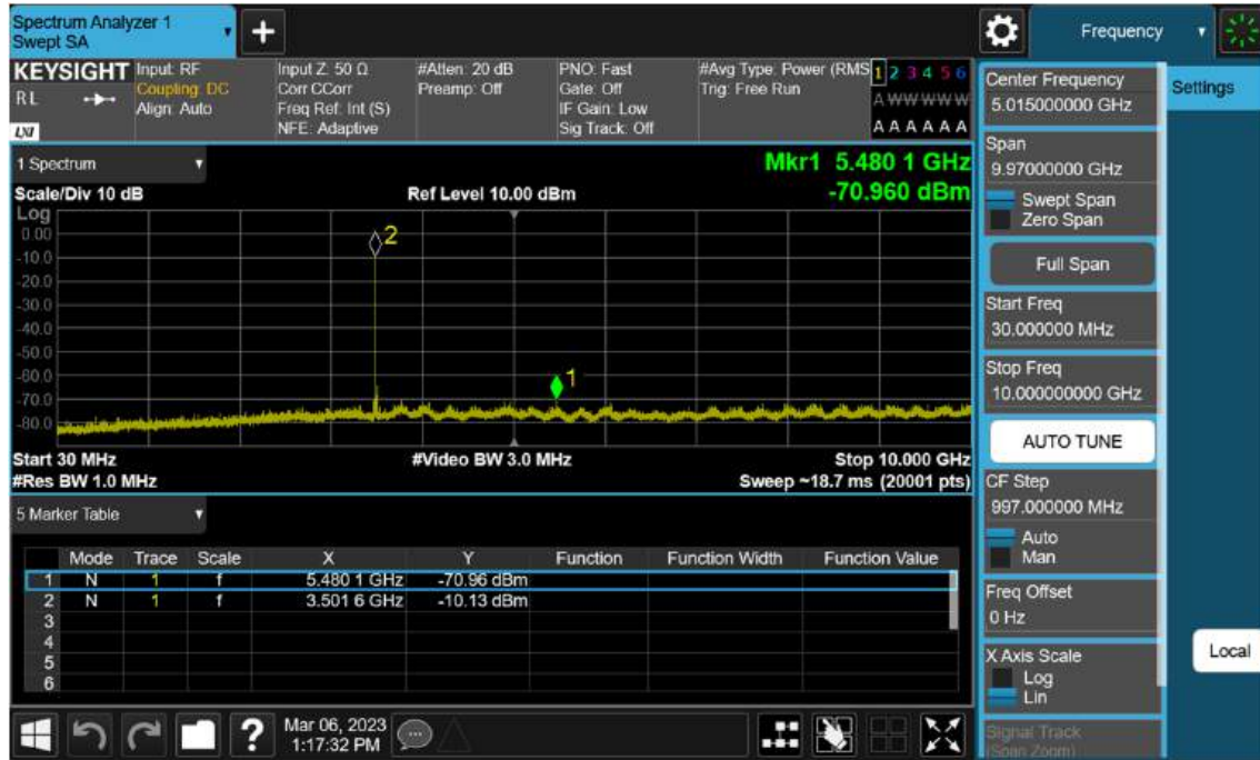
Sub6 n77(78). Conducted Spurious Plot_1 (635000ch_50 MHz_BPSK)
