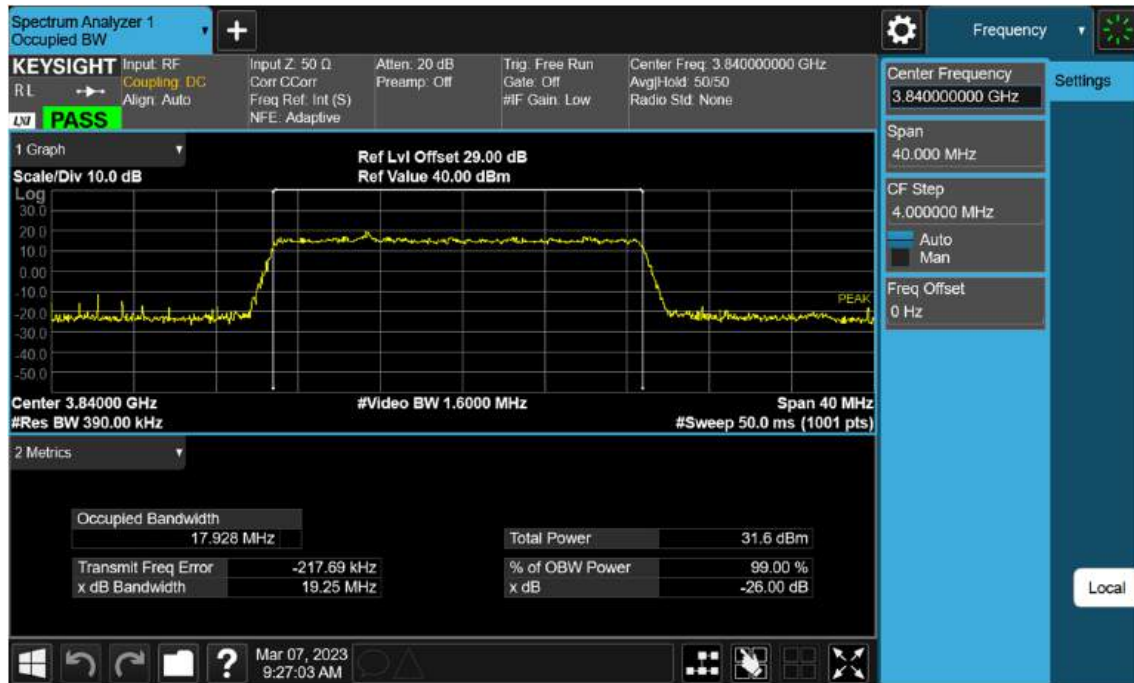
Sub6 n77(78). Occupied Bandwidth Plot (20 M BW Ch.656000 BPSK )
