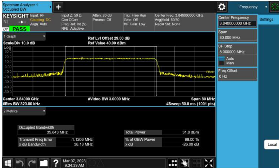
Sub6 n77(78). Occupied Bandwidth Plot (40 M BW Ch.656000 QPSK )
