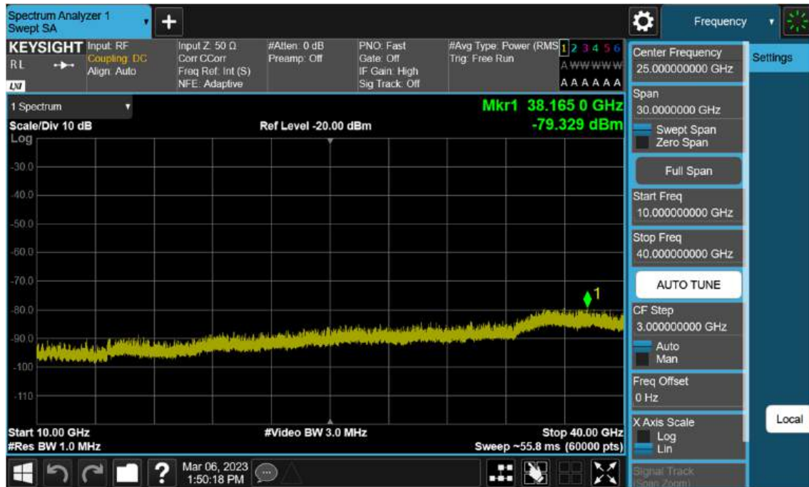
Sub6 n77(78). Conducted Spurious Plot_2 (633334ch_80 MHz_BPSK)
