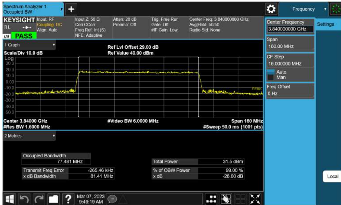
Sub6 n77(78). Occupied Bandwidth Plot (80 M BW Ch.656000 16QAM )
