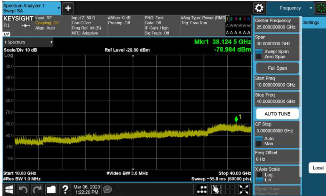
Sub6 n77(78). Conducted Spurious Plot_2 (632000ch_60 MHz_BPSK)
