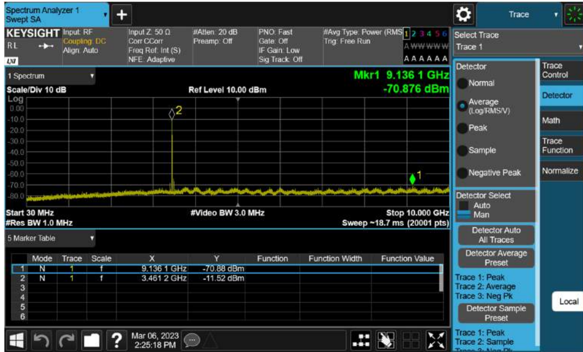
Sub6 n77(78). Conducted Spurious Plot_1 (633666ch_90 MHz_BPSK)
