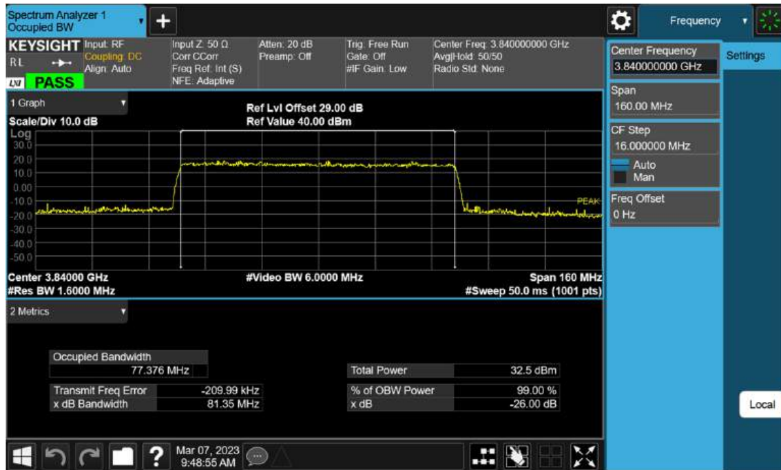
Sub6 n77(78). Occupied Bandwidth Plot (80 M BW Ch.656000 QPSK )
