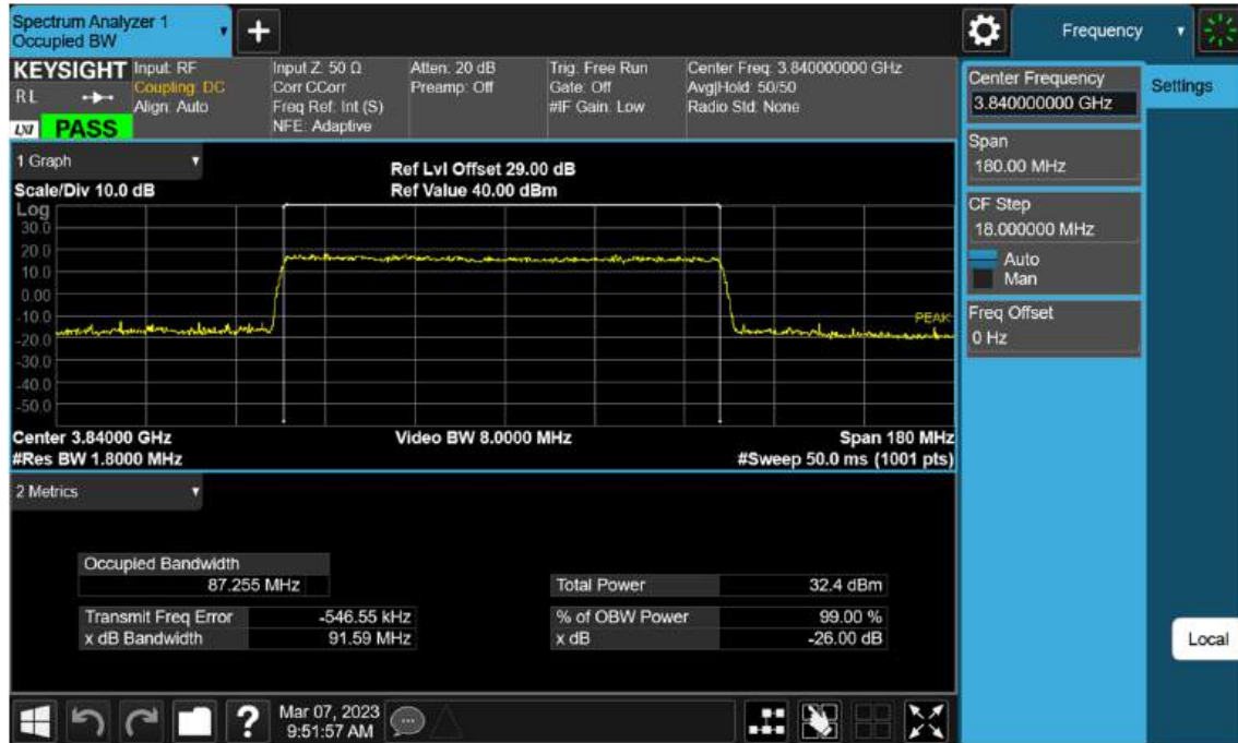
Sub6 n77(78). Occupied Bandwidth Plot (90 M BW Ch.656000 QPSK )
