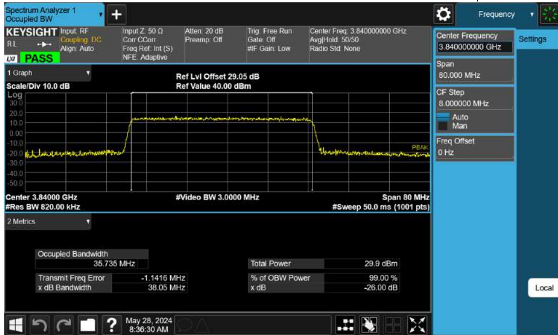
Sub6 n77(78). Occupied Bandwidth Plot (40 M BW Ch.656000 256 QAM )
