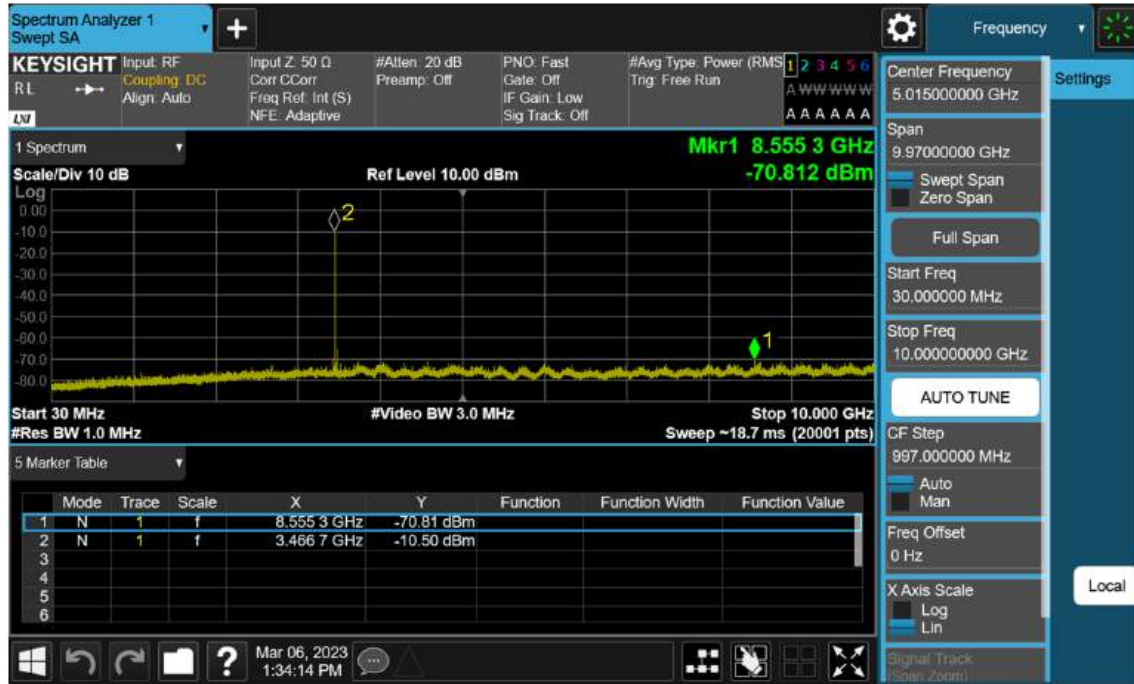
Sub6 n77(78). Conducted Spurious Plot_1 (633334ch_70 MHz_BPSK)
