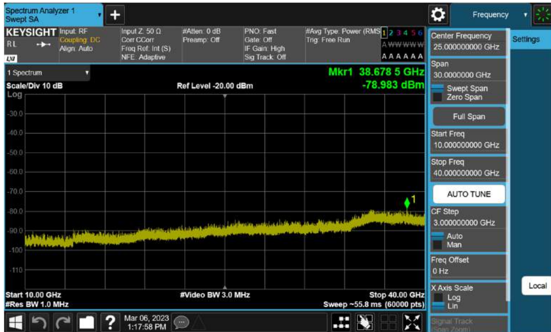
Sub6 n77(78). Conducted Spurious Plot_2 (635000ch_50 MHz_BPSK)
