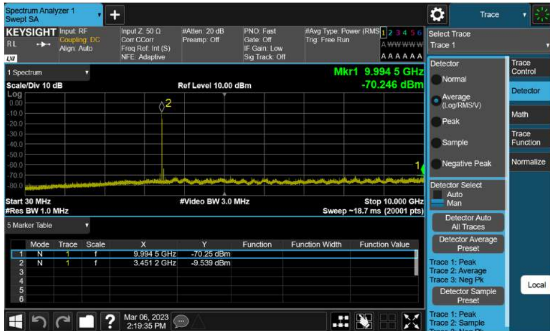
Sub6 n77(78). Conducted Spurious Plot_1 (633000ch_90 MHz_BPSK)
