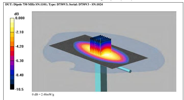
Communication System: CW 750; Frequency: 750 MHz; Duty Cycle: 1:1
