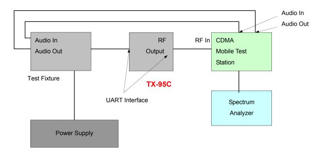
UART Interface: The UART Interface has a serial communication link and RF Interface port that can be used to test, debug or upgrade the phone's functions and characteristics.
