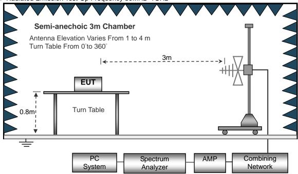
(C) Radiated Emission Test-Up Frequency Above 1GHz
