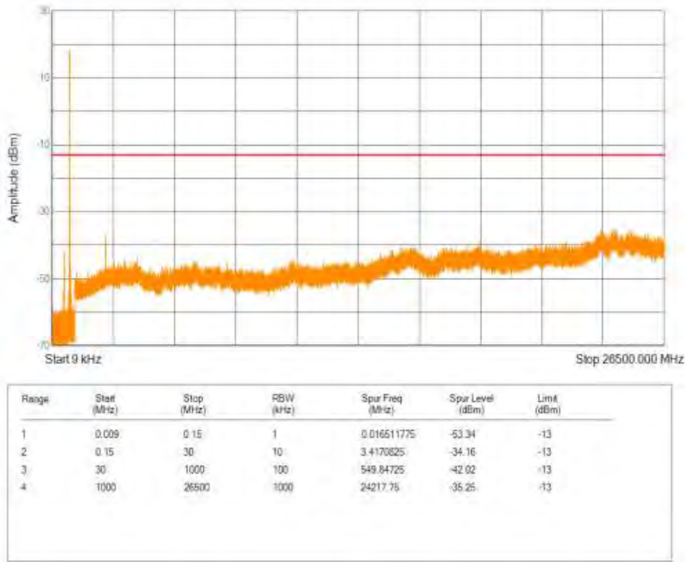
Band13 16QAM BW=5MHz Channel=23230 RB Size=1 Position=#0 NB Index=0
