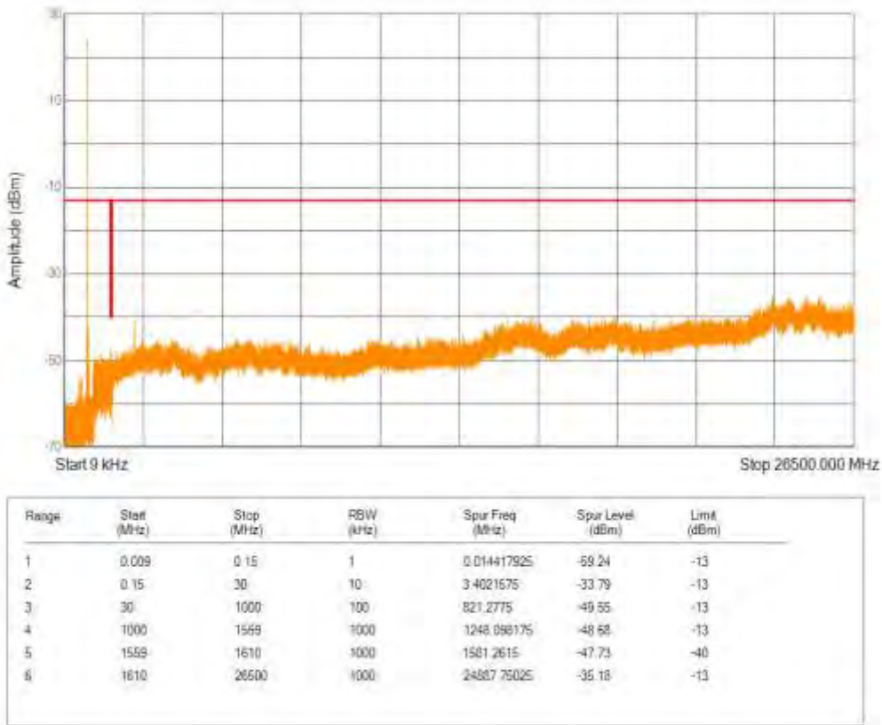
Band14 16QAM BW=5MHz Channel=23330 RB Size=5 Position=#0 NB Index=0
