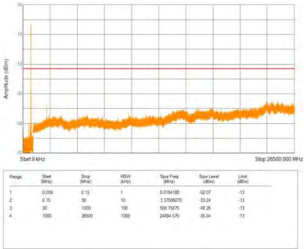
Band13 16QAM BW=5MHz Channel=23255 RB Size=1 Position=#0 NB Index=0
