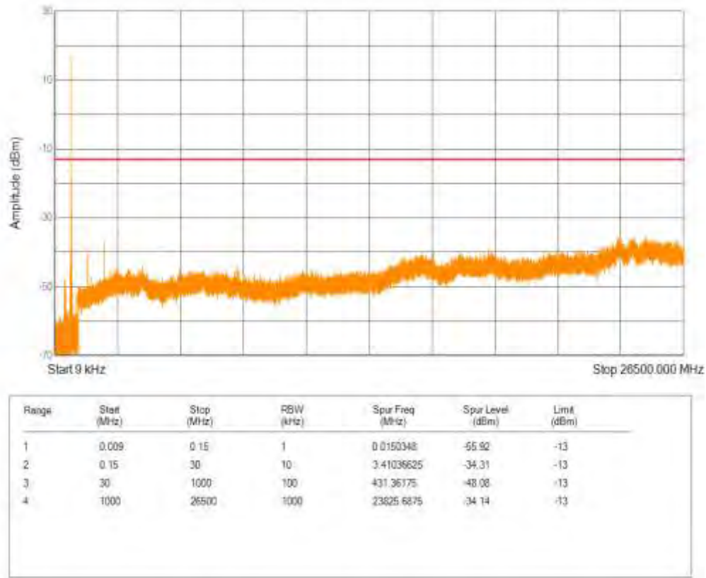
Band12 16QAM BW=10MHz Channel=23060 RB Size=1 Position=#0 NB Index=0
