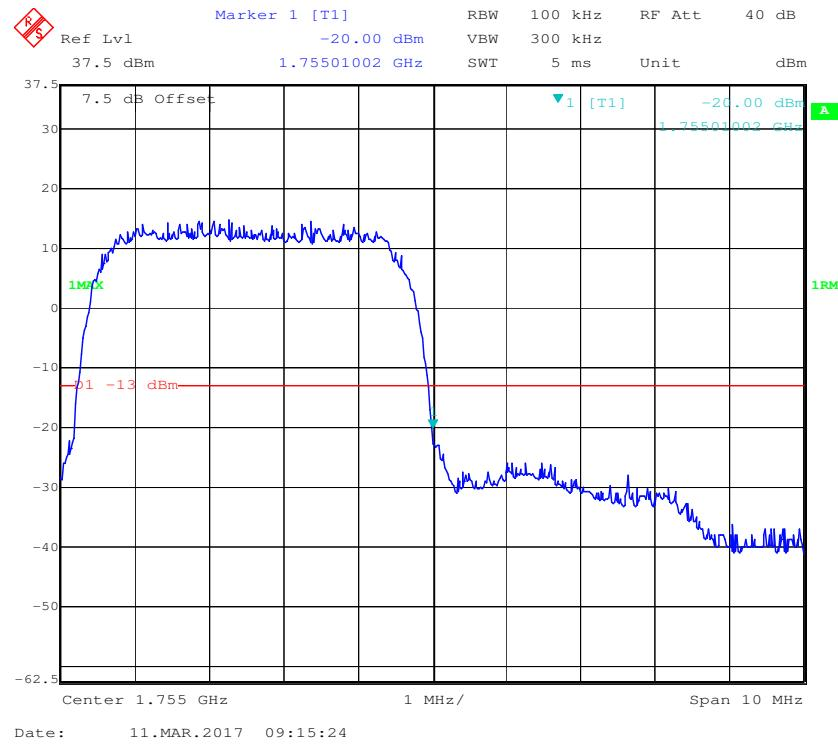
**AWS Band, Left Band Edge for HSDPA (16QAM) Mode**
