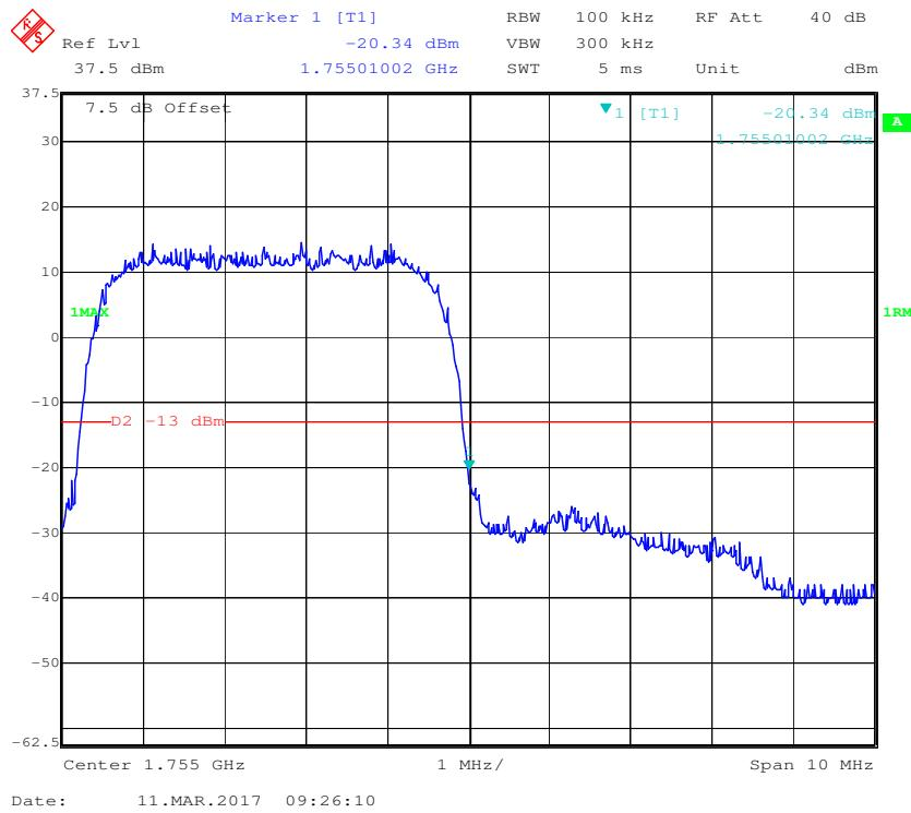
**AWS Band, Left Band Edge for HSUPA (BPSK) Mode**
