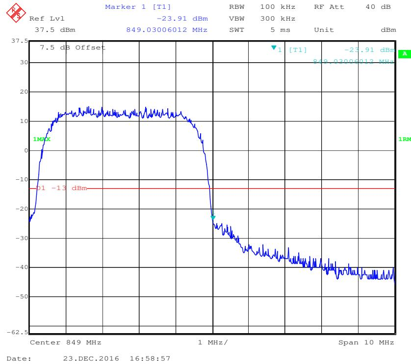
**PCS Band, Left Band Edge for GSM (GMSK) Mode**
