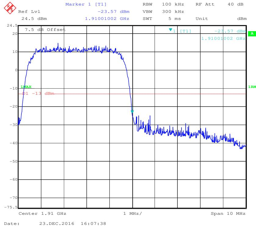
**PCS Band, Left Band Edge for HSUPA (BPSK) Mode**
