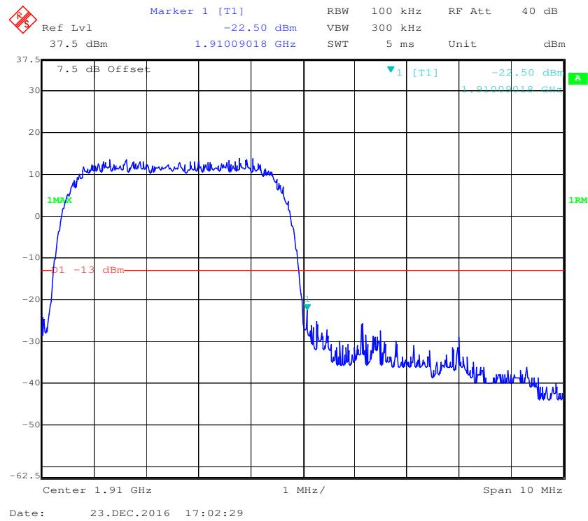
**AWS Band, Left Band Edge for WCDMA (BPSK) Mode**
