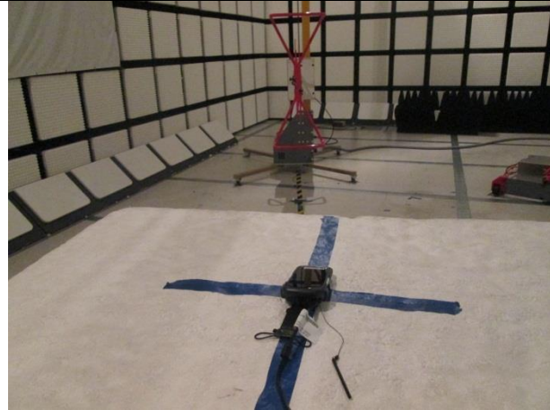
RADIATED FRONT PHOTO (BELOW 1 GHz)
