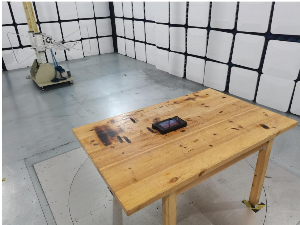
Photo of Radiation Emission Test
