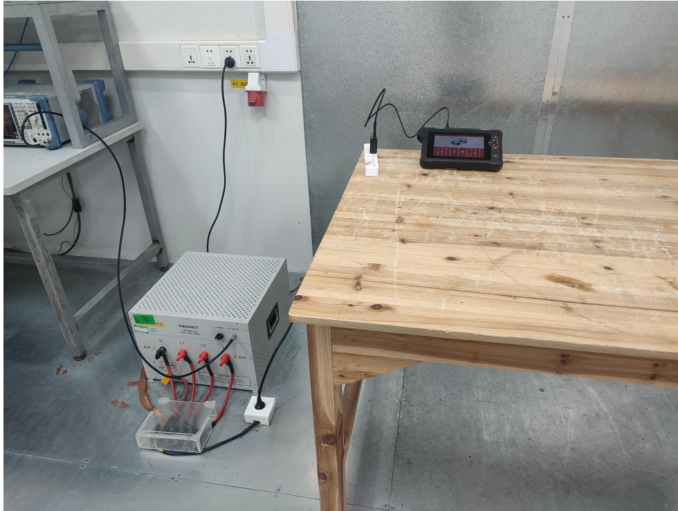
Photo of Power Line Conducted Emission Test
