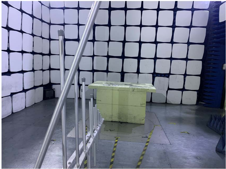
Radiation Emission Test Setup (30MHz to 1GHz)
